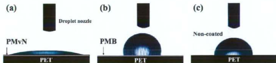
Figure 5. Water droplets on the surfaces under dry condition after contact for 2 s: (a) PMvN-coated PET, (b) PMB-coated PET, (c) noncoated PET.
