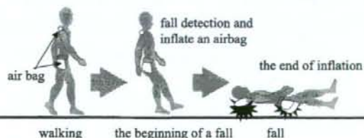
Fig.1 Schematic diagram of inflating the air bag
