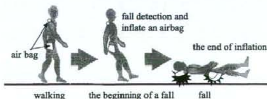
Fig.1 Schematic diagram of inflating the air bag
