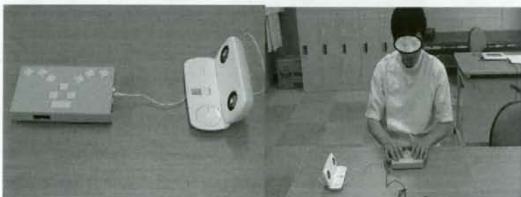
Fig. 4. Note-taking tool in Braille-typewriter mode "L. L. Writer"
