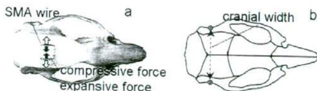
Fig. 1. a SMA wire applying compressive and expansive forces on the rat cranium. b Schema demonstrating the dimension assessed on soft X-ray photographs
