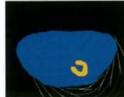
Fig. 2. The orbits of the detector according to the rotating angles. White lines are the orbits of detector. The rotating angle is  $180^\circ$  for the outermost orbit. The rotating angle is  $45^\circ$  for the innermost orbit.
