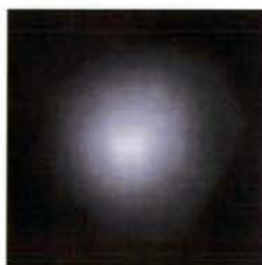
Fig. 2. Output beam spatial structure of 1.06 \mu\text{m} Nd:YAG laser radiation (2D image, Electrim CCD camera EDC-1000HR).
