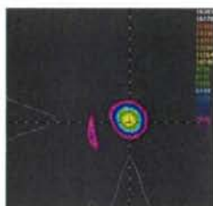
Fig. 6. Output beam spatial structure of 1.34 \mu\text{m} Nd:YAG laser radiation behind waveguide with 100 \mu\text{m} inner diameter and 10 cm length (2D and 3D image - pyroelectric camera Spiricon Pyrocam III).
