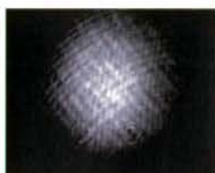
Fig. 3. Output beam spatial structure of 1.06 \mu\text{m} Nd:YAG laser radiation behind waveguide with 100 \mu\text{m} inner diameter and 10 cm length (2D image, Electrim CCD camera EDC-1000HR).
