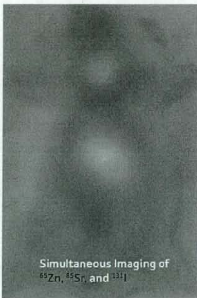
Figure 1: Compound image from a Compton camera showing the positions of three different radioisotopes, zinc (red), strontium (blue) and iodine (green), in a live mouse. (This work was completed in compliance with Japan's ethical standards for experiments on live animals.)
