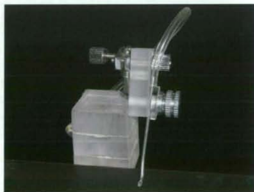
Figure 4 | A custom-made holder for the outlet needle (Narishige). Height, rotation angle and lean angle of the needle are freely adjustable without using a screwdriver.
