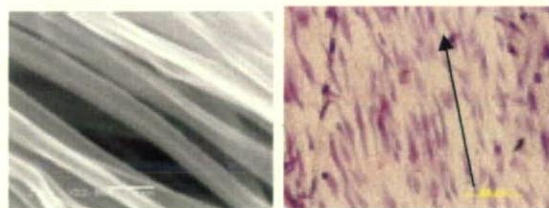
(a) SEM Image of aligned PVA nanofibers
