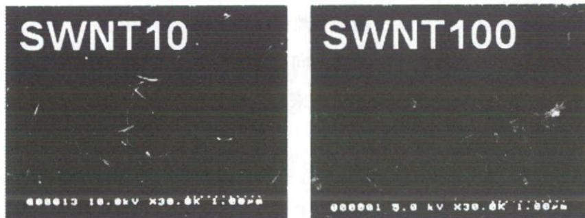
Fig 1. SEM images of SWNT conductive thin film on PS dish (SWNT10: 10 $\mu$ gCNTs/6cm dish, SWNT100: 100 $\mu$ gCNT/6cm dish)
