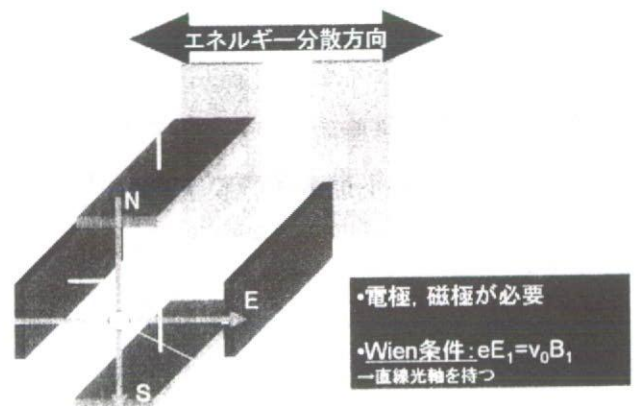
Figure 2 Principle of Wien filter.
