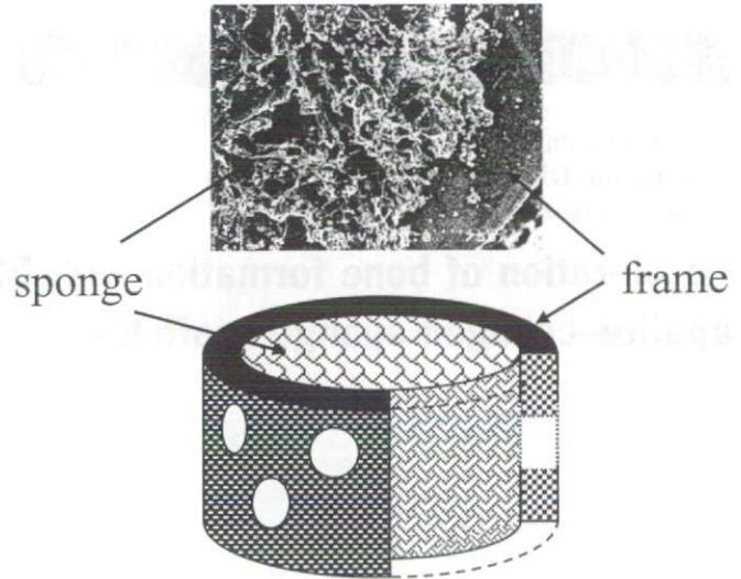
Fig. 1. Sponge reinforced with a hydroxyapatite (Hap) frame
