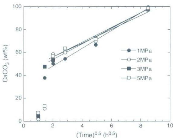
**Fig. 5** Changes in the amount of calcite phase in the compacts plotted against square root of time with time at various molding pressures
