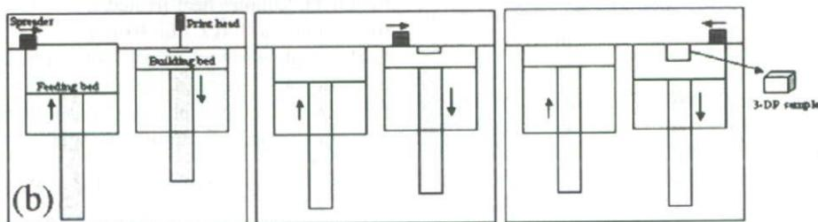
Figure 2. (a) 3DP machine (Z310, Z Corporation); (b) fabrication process of 3DP system.
