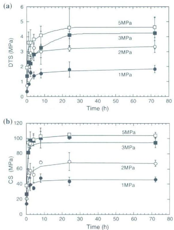
**Fig. 6** (a) Changes in diametral tensile strength of compacts pressed at 1, 2, 3 and 5 MPa during carbonation with time. (b) Changes in compressive strength of column compacts pressed at 1, 2, 3 and 5 MPa during carbonation with time
