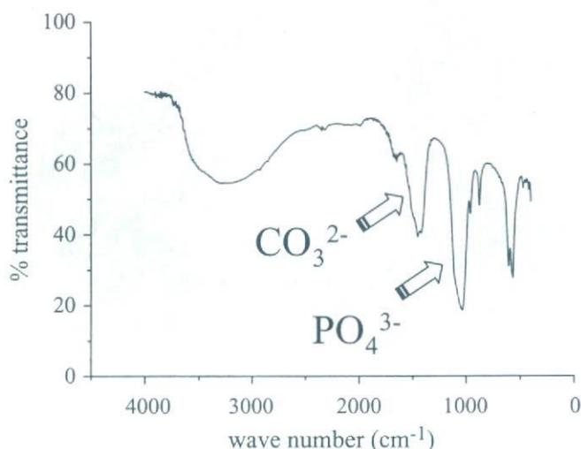
**Fig. 3.** Fourier transform infrared spectroscopy (FT-IR) spectrum of  $\text{CO}_3\text{Ap}$
