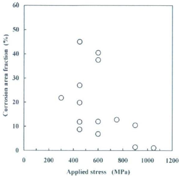
**Figure 3.** Fraction of corrosion area on fracture surface as function of applied stress.
