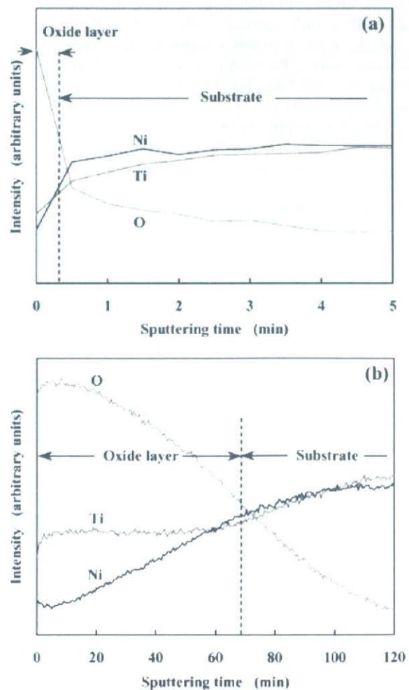
**Figure 9.** Typical AES depth profile of (a) nonimmersed specimen and (b) specimen immersed in physiological saline solution containing hydrogen peroxide without applied stress for 24 h.
