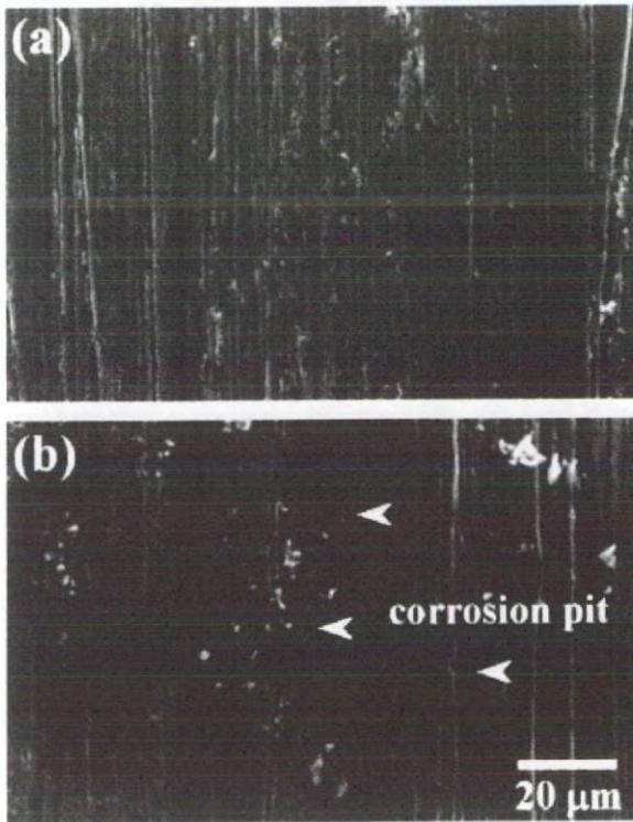
Figure 6. SEM images of side surface of (a) nonimmersed specimen and (b) specimen immersed in physiological saline solution containing hydrogen peroxide without applied stress for 120 h.
