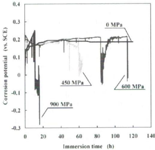
Figure 5. Changes in corrosion potential for various applied stresses in physiological saline solution containing hydrogen peroxide.
