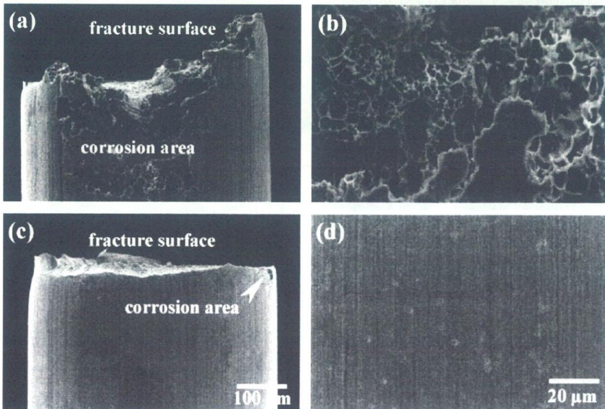
**Figure 4.** SEM images of typical side surface after sustained tensile-loading test in physiological saline solution containing hydrogen peroxide under applied stress of 450 MPa, (a) general and (b) magnified views; and under applied stress of 900 MPa, (c) general and (d) magnified views.
