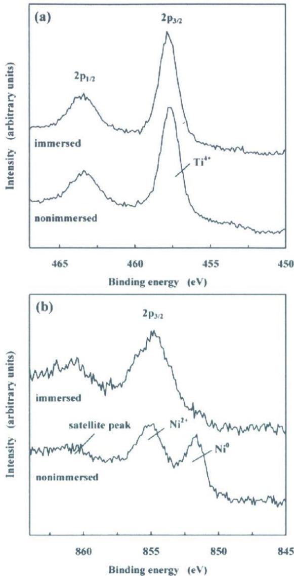
**Figure 8.** Typical XPS spectra of nonimmersed specimen and specimen immersed in physiological saline solution containing hydrogen peroxide without applied stress for 24 h: (a) Ti 2p and (b) Ni 2p<sub>3/2</sub>.
