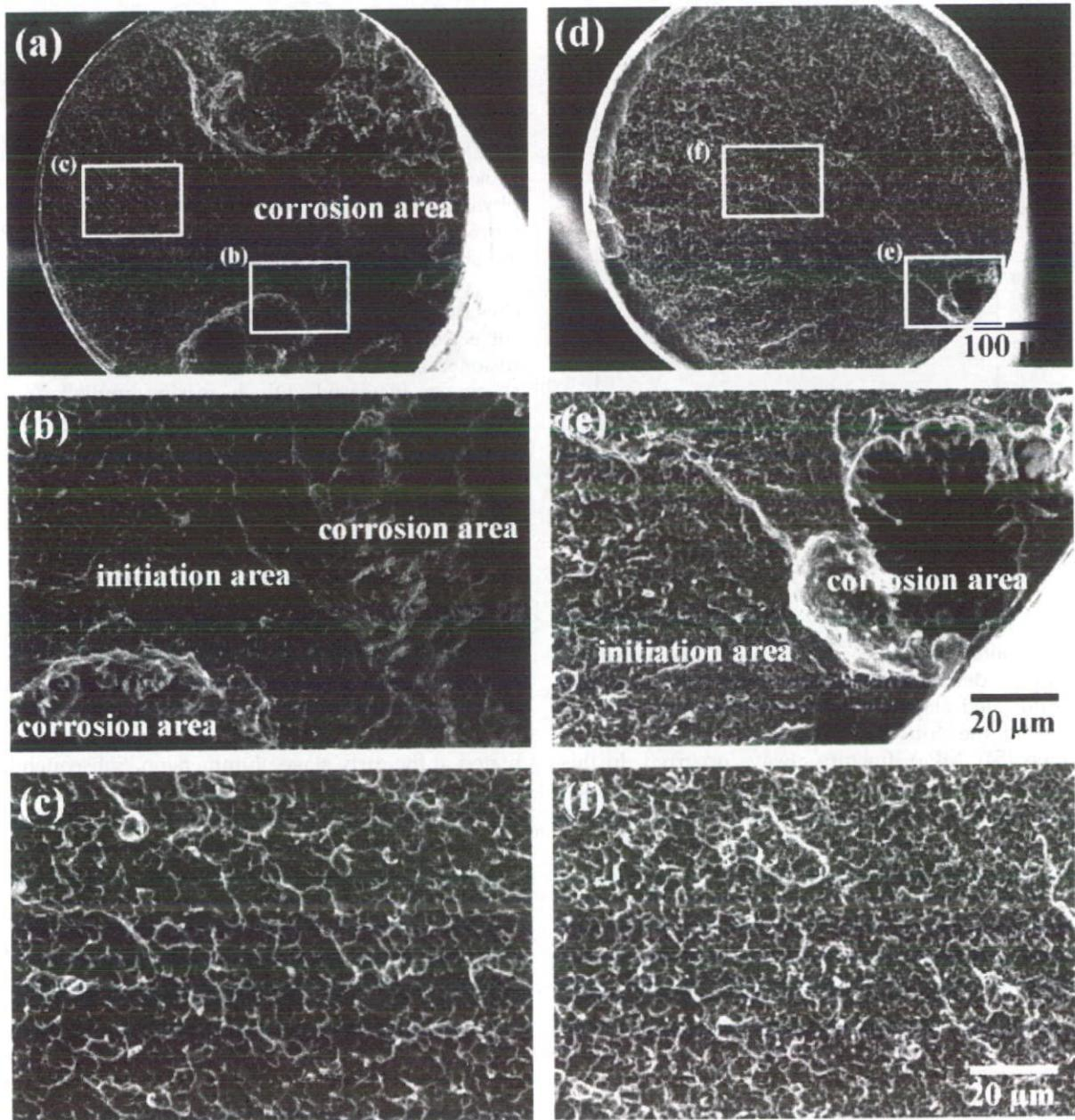
**Figure 2.** SEM images of typical fracture surface after sustained tensile-loading test in physiological saline solution containing hydrogen peroxide; (a) under applied stress of 450 MPa, (b) fracture initiation area and (c) crack propagation area, and (d) under applied stress of 900 MPa, (e) fracture initiation area and (f) crack propagation area.
