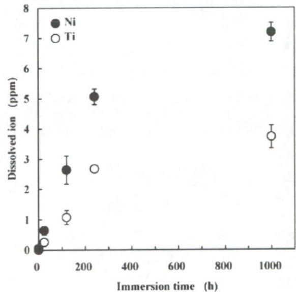
Figure 7. Amounts of dissolved nickel and titanium ions immersed in physiological saline solution containing hydrogen peroxide without applied stress.
