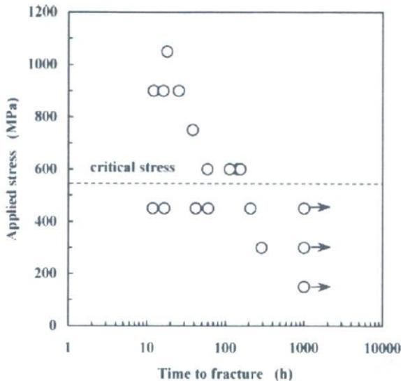
**Figure 1.** Time to fracture versus initial applied stress for Ni-Ti superelastic alloy immersed in physiological saline solution containing hydrogen peroxide.
