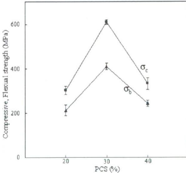
**Figure 4.** Compressive strength  $\sigma_c$  and flexural strength  $\sigma_b$  of the sintered MWCNTs.
