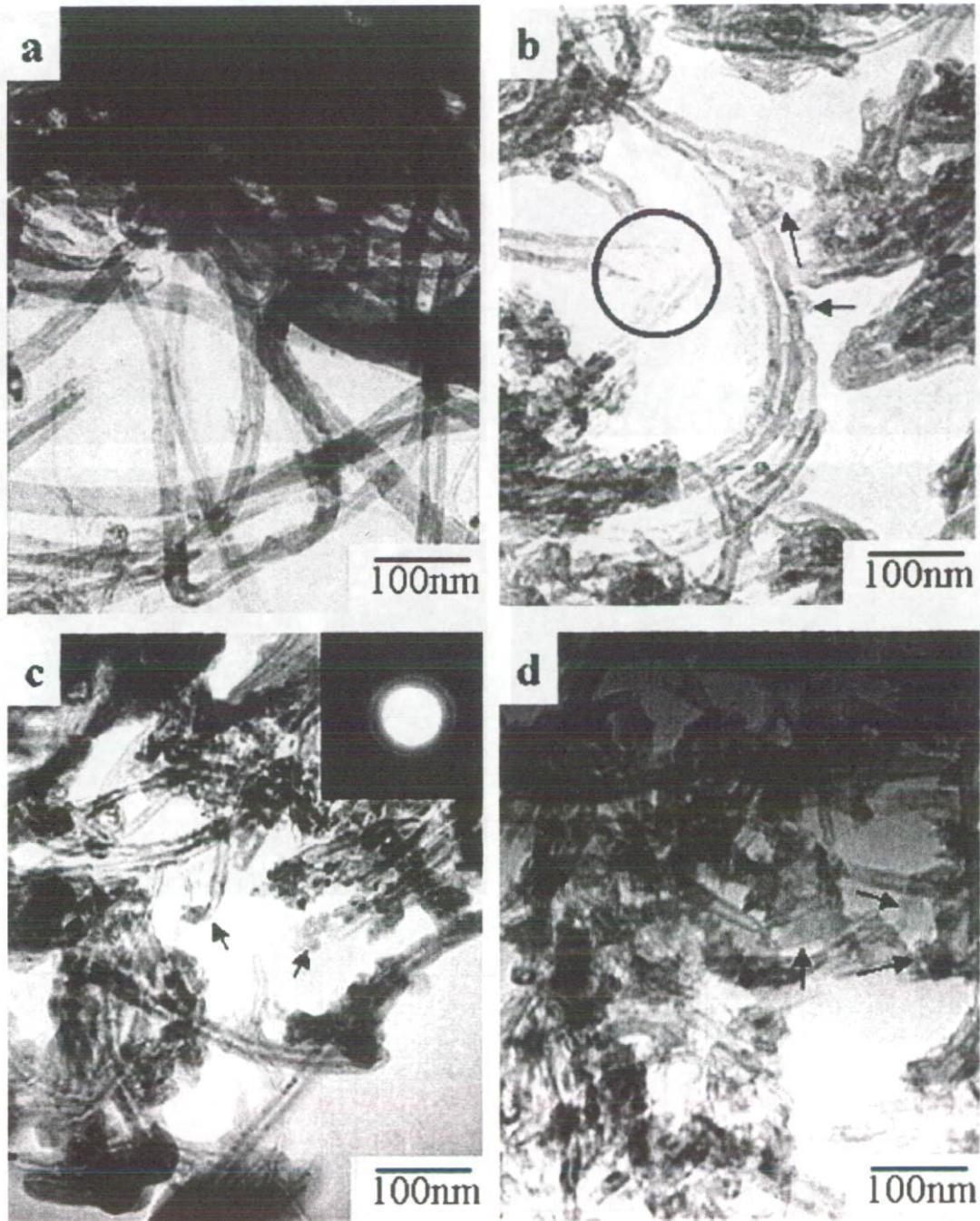
**Figure 7.** TEM images of MWCNT powders (a), MWCNT/20% PCS (b), MWCNT/30% PCS (c), and MWCNT/40% PCS (d).
