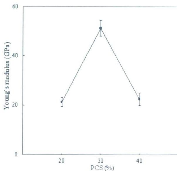
Figure 3. Dependence of Young's modulus of the sintered MWCNTs on PCS content.
