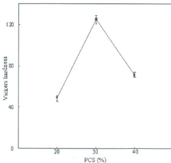
Figure 2. Dependence of Vickers hardness of the sintered MWCNTs on PCS content.
