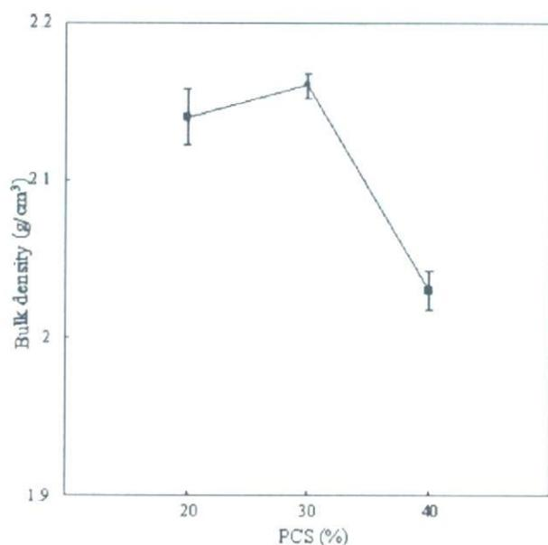
Figure 1. Dependence of bulk density of the sintered MWCNTs on PCS content.
