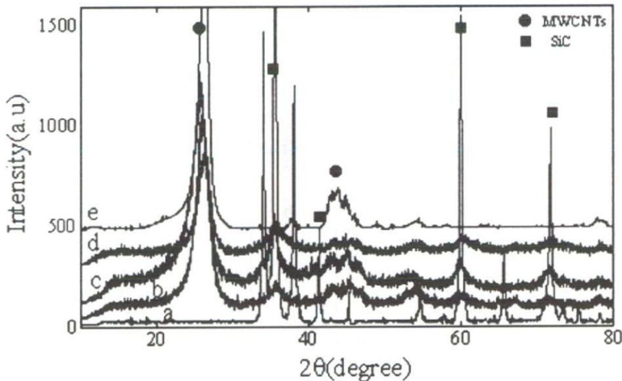
**Figure 5.** XRD patterns of sintered MWCNTs with 20% PCS (b), 30% PCS (c), and 40% PCS (d), compared with MWCNT powders (e) and SiC powders (a).
