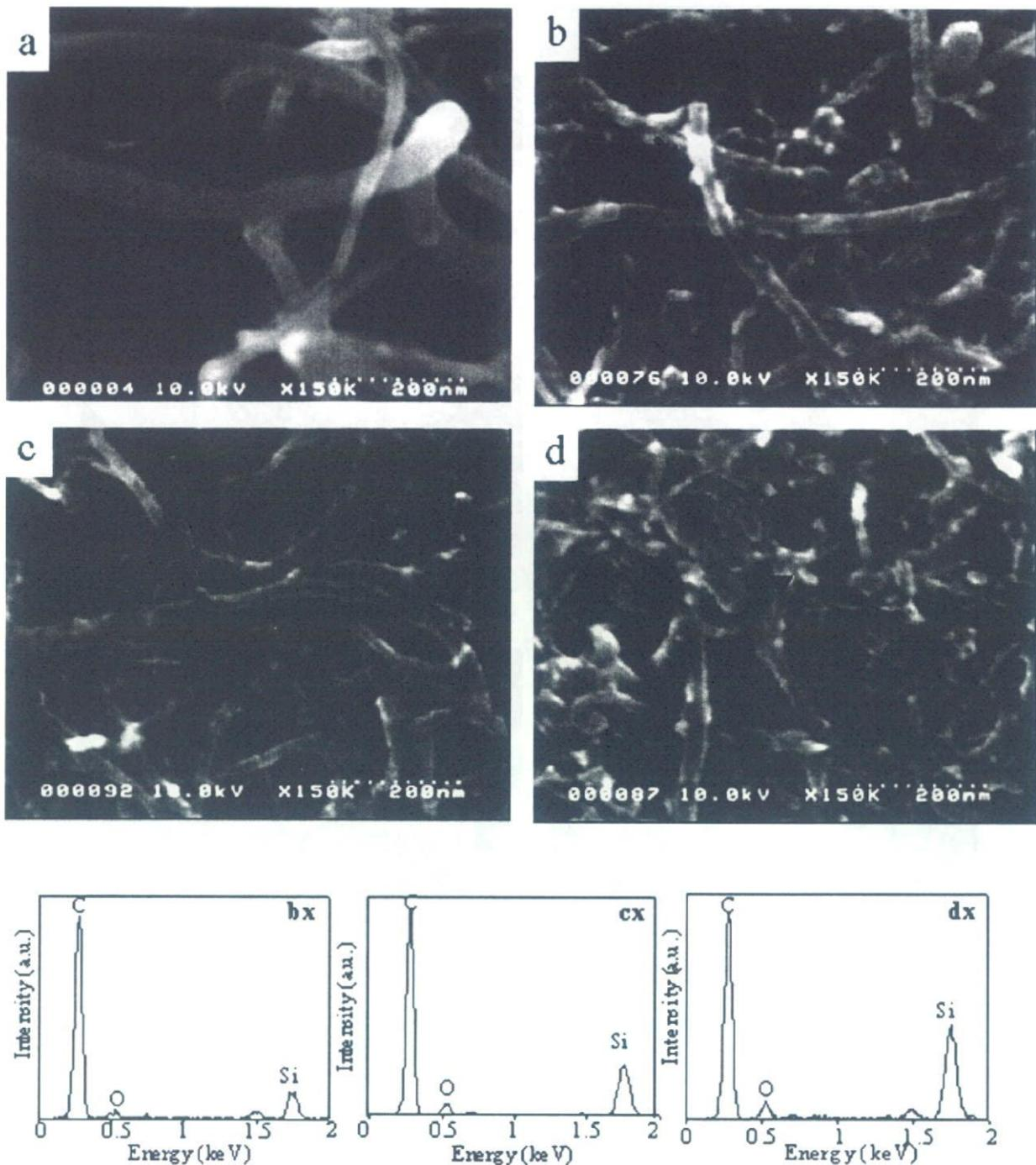
**Figure 6.** SEM images and corresponding EDS analyses of MWCNTs before sintering (a), MWCNT/20% PCS (b), (bx); MWCNT/30% PCS (c), (cx); and MWCNT/40% PCS (d), (dx).
