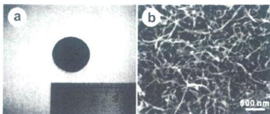
**FIGURE 1.** (a) Typical image of condensed-MWCNT films. (b) SEM image of the surface of condensed-MWCNT films.
