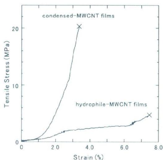
**FIGURE 5.** Tensile stress-strain curves of hydrophile-MWCNT and condensed-MWCNT films.
