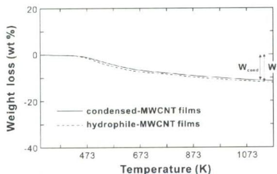
**FIGURE 4.** TG curves of hydrophilic-MWCNT (dashed line) and condensed-MWCNT (solid line) films. *W<sub>h</sub>* and *W<sub>cond</sub>* represent the decreasing weight percentage of hydrophilic-MWCNT and condensed-MWCNT films, respectively, at 1173K.
