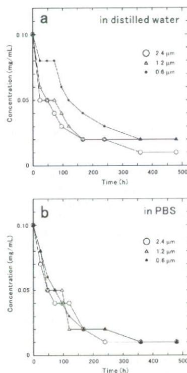
**FIGURE 5.** Stability of size-separated CNFs in distilled water (a) and PBS (b).
