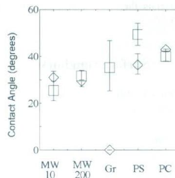
FIGURE 2. Contact angle of the surface of each scaffold material. □: soaked in deionized water and ◇: soaked in PBS(-).
