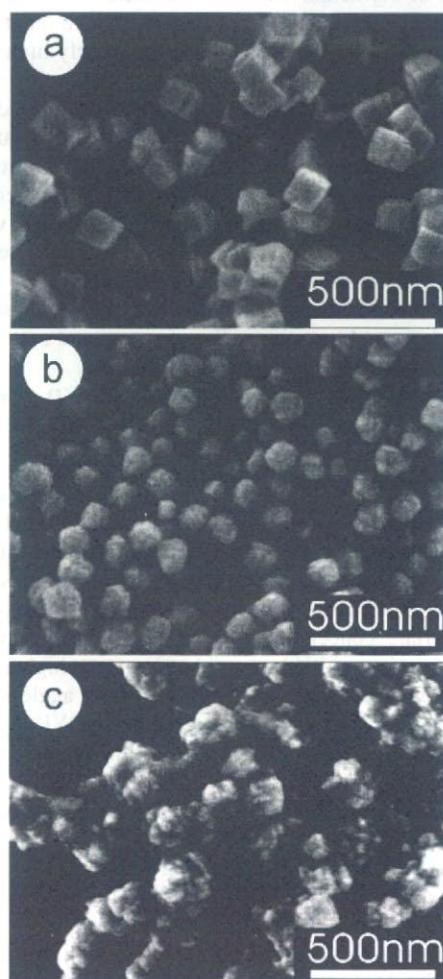
FIGURE 2. SEM images of (a) Fe<sub>75</sub>Co<sub>25</sub> and (b) Fe<sub>50</sub>Co<sub>50</sub>, and Fe<sub>75</sub>Co<sub>25</sub> particles synthesized with surfactant, and (c) the FeCo particles prepared in the absence of surfactant.
