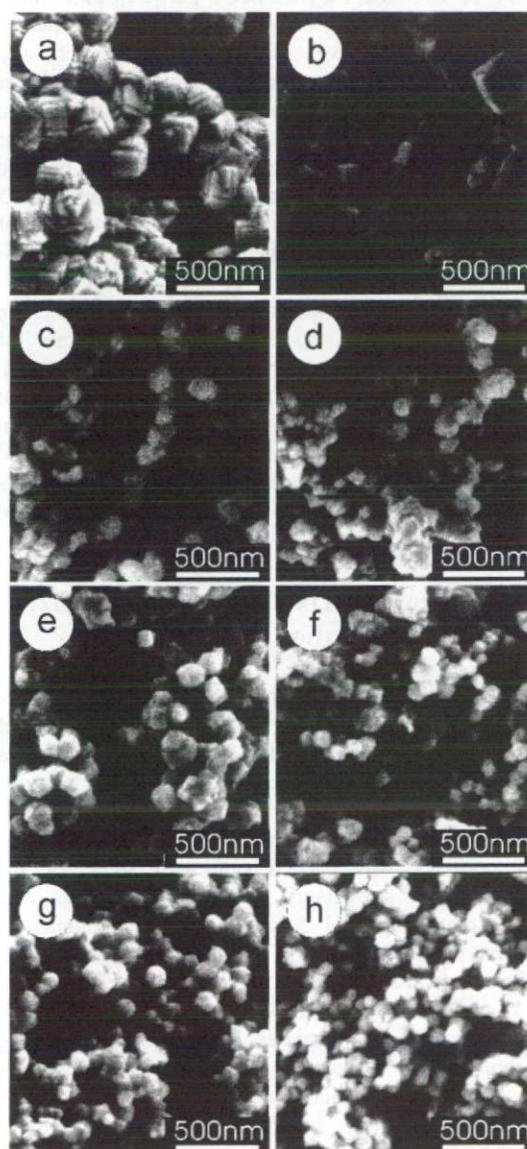
**FIGURE 3.** SEM image of the FeCo particles synthesized with surfactant (a) oleylamine, surfactant / metal molar ratio (S / M) = 1, (b) oleylamine S / M = 10, (c) oleic acid, (d) stearic acid, (e) lauric acid, (f) adamantane carboxylic acid, (g) sodium dodecyl benzene sulfonate and (h) PVP K-16.
