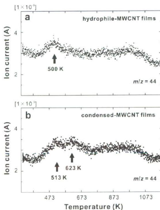
**FIGURE 3.** Generation of CO<sub>2</sub> (*m/z* 44) of (a) hydrophilic-MWCNT and (b) condensed-MWCNT films in a helium atmosphere.
