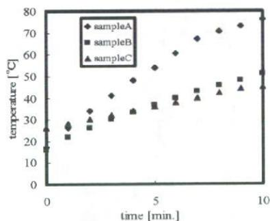
FIGURE 2. Temperature against exposure time of the magnetite suspensions dispersing samples A, B and C exposed to an ac magnetic field. (intensity 3.2 kA/m and frequency 600 kHz)
