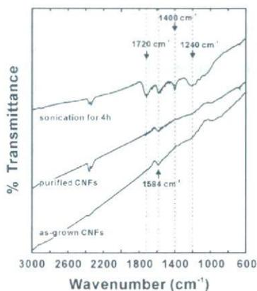
FIGURE 3. IR spectra of H-CNFs. From bottom: as-grown, purified, and cut H-CNFs.
