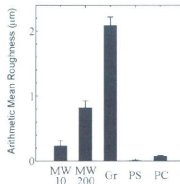
FIGURE 3. Surface roughness of each scaffold material.
