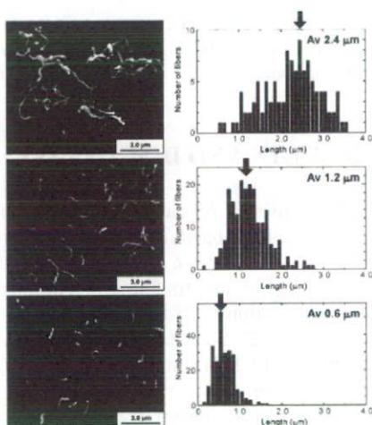
**FIGURE 4.** SEM images of cake on a filter (left) and corresponding size-distributions (right) of separated H-CNFs.
