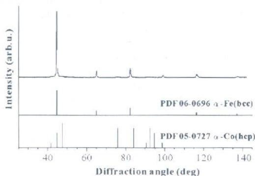
FIGURE 1. XRD pattern of FeCo particles synthesized by modified polyol process.
