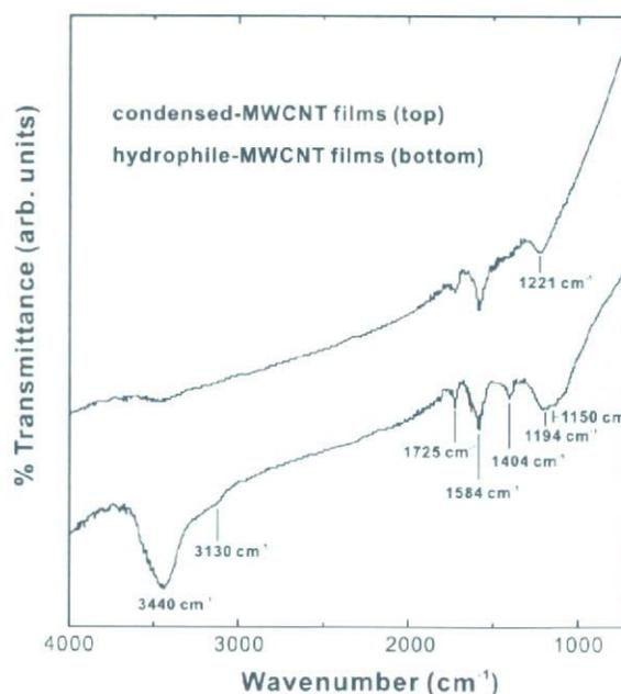
**FIGURE 2.** FT-IR spectra of condensed-MWCNT films (top), and hydrophile-MWCNT films (bottom).
