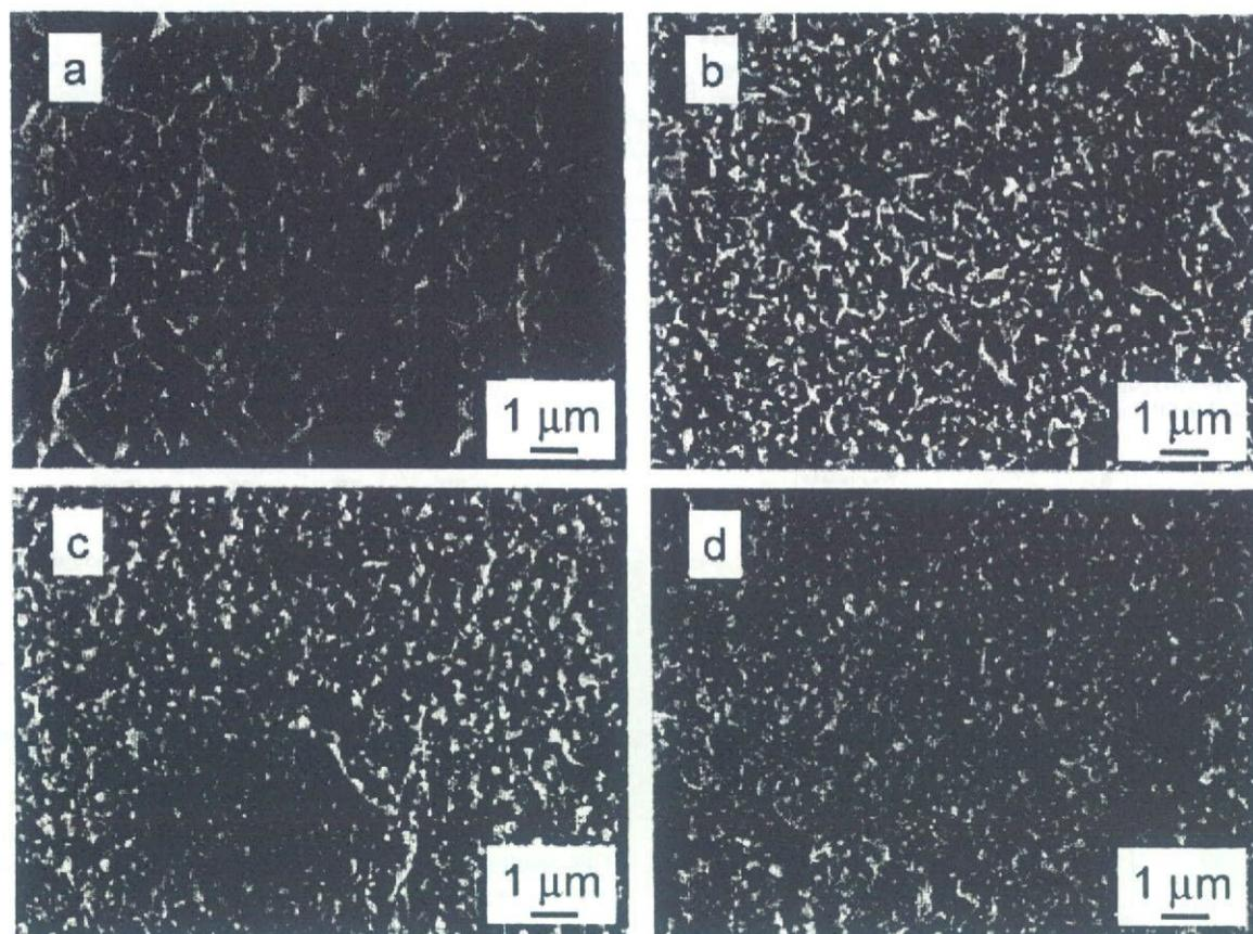
Fig. 3 Scanning electron micrographs of fracture surfaces of TiO<sub>2</sub>/HDPE composites –20 (a), 40 (b), 52 (c) and 55.6 vol% (d)
