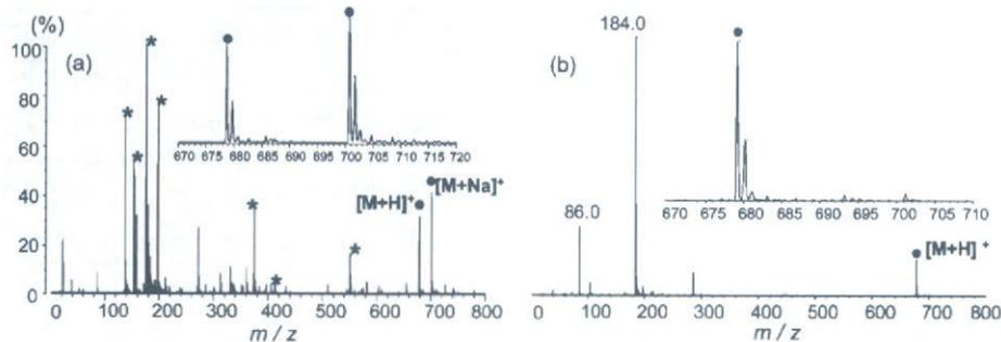
**Figure 5.** The mass spectra of DMPC (0.2 mg/mL, 0.5 mL) obtained from (a) DHB matrix for MALDI-MS and (b) Pt nanoflowers for SALDI-MS. Characteristic matrix signals are marked with asterisks.
