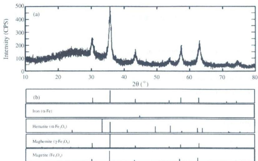
Fig. 5. (a) XRD pattern of iron oxide nanoparticles stabilized by gelatin. (b) Diffraction peaks extracted from pattern in (a) ( $\text{FeCl}_3 \cdot 6\text{H}_2\text{O}$ : 175 mg).
