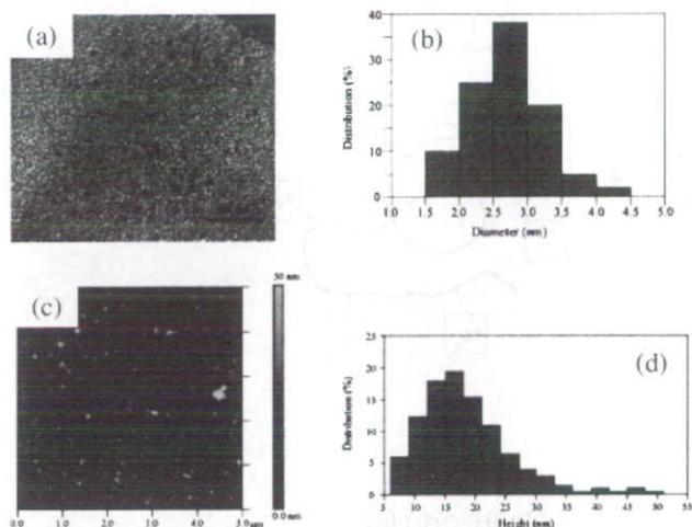
Fig. 3. (a) TEM image of gelatin-stabilized iron oxide nanoparticles and (b) their size distribution. (c) AFM image of gelatin-stabilized iron oxide nanoparticles placed on a graphite substrate and (d) the height distribution of particles ( $\text{FeCl}_3 \cdot 6\text{H}_2\text{O}$ : 175 mg).
