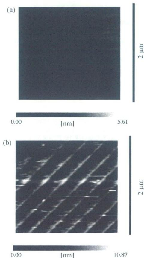
Fig. 3. AFM images of (a) the nanoline patterns prepared on a Si wafer covered by TTCl-SAM and (b) the modified nanolines on the TTCl-SAM coated silicon wafer after immersion into Ag nanoparticle dispersion.
