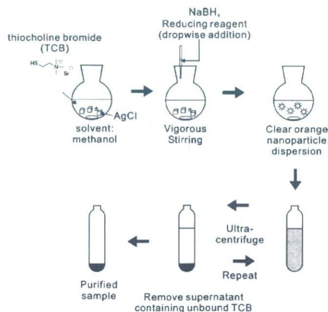
Fig. 1. Schematic illustration of preparation and purification of cationic Ag nanoparticles stabilized by thiocholine bromide.
