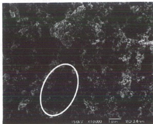
**Figure 8.** HR-SEM images of the surface of the Pt nanoflower SALDI-MS plates after laser irradiation.
