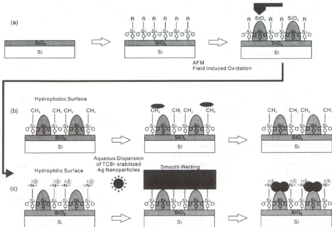
Fig. 2. Schematic illustration of FIO (field induced oxidation) lithography with a scanning probe (a). Immobilization of cationic Ag nanoparticles onto oxide area prepared on (b) OTS-SAM or (c) TTCl-SAM.
