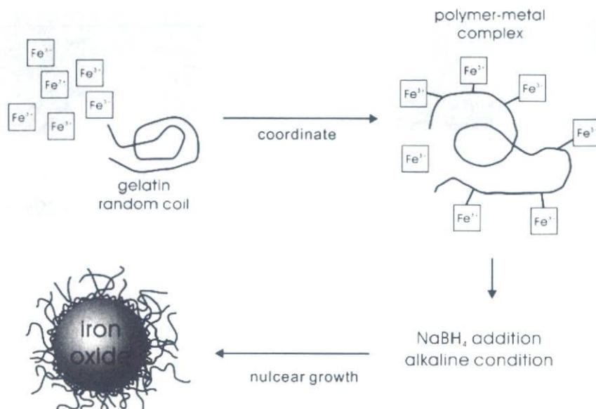
Fig. 1. Schematic illustration of preparation procedure of iron oxide nanoparticles stabilized by gelatin molecules.
