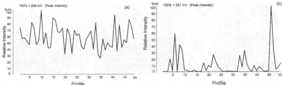
**Figure 3.** Plot of relative peak intensities of angiotensin I (500 fmol) obtained from 50 different sample spots in SALDI-MS with (a) Pt nanoflowers and (b) DHB matrix (15 mg/mL). The conditions for Pt nanoflowers were the same as those in Figure 2. In the case of DHB, the sample data were collected at the edges of the sample, which might be sweet-spot positions.
