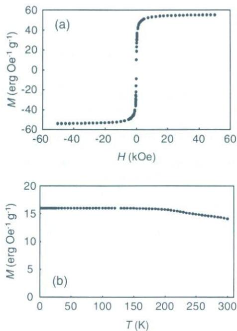
Fig. 6. (a) Hysteresis curve and (b) ZFC curve of the obtained iron oxide nanoparticles ( $\text{FeCl}_3 \cdot 6\text{H}_2\text{O}$ : 175 mg).
