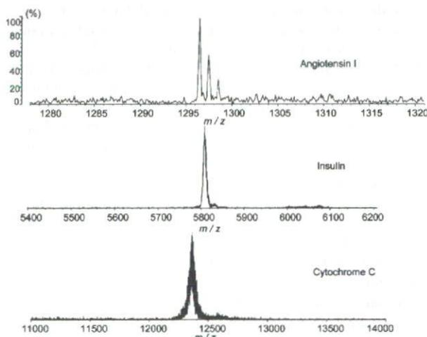
**Figure 4.** The mass spectra of (a) angiotensin I (0.7 fmol), (b) human insulin (5 fmol), and (c) cytochrome C (20 fmol) obtained from Pt nanoflowers for SALDI-MS.
