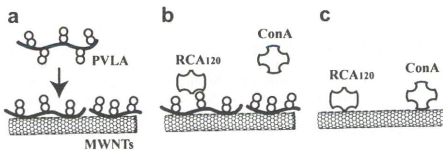
**Scheme 1.** Illustrations of (a) adsorption of PVLA onto the surface of MWNTs, (b) specific interaction between the MWNTs coated with PVLA and lectins, and (c) non-specific interaction between MWNTs and lectins.
