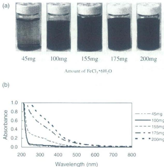
Fig. 2. (a) Images of the dispersion of gelatin-stabilized magnetic nanoparticles with various iron concentrations, and (b) UV-vis spectra of these dispersions.
