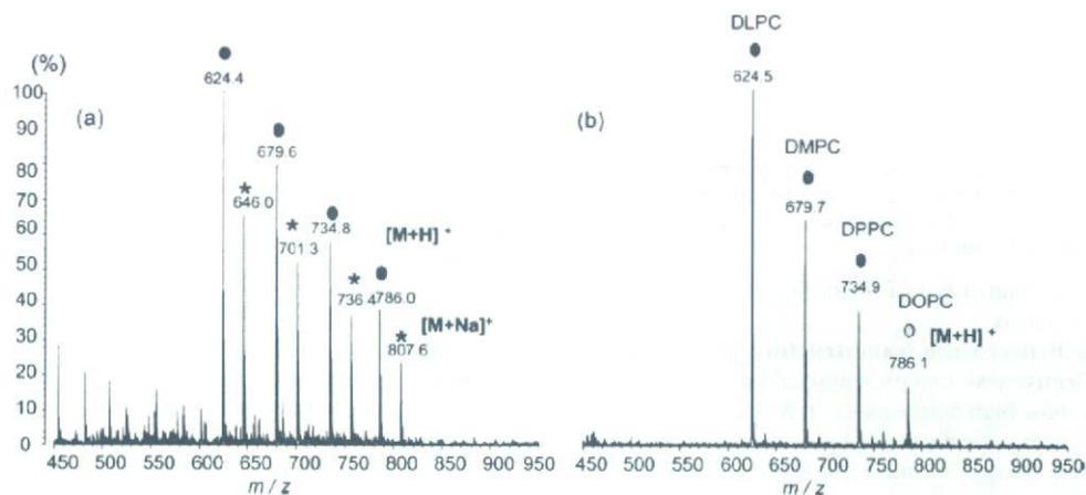
**Figure 6.** The mass spectra of the lipid mixtures of DLPC, DMPC, DPPC, and DOPC with (a) DHB matrix for MALDI-MS and (b) Pt nanoflowers for SALDI-MS.
