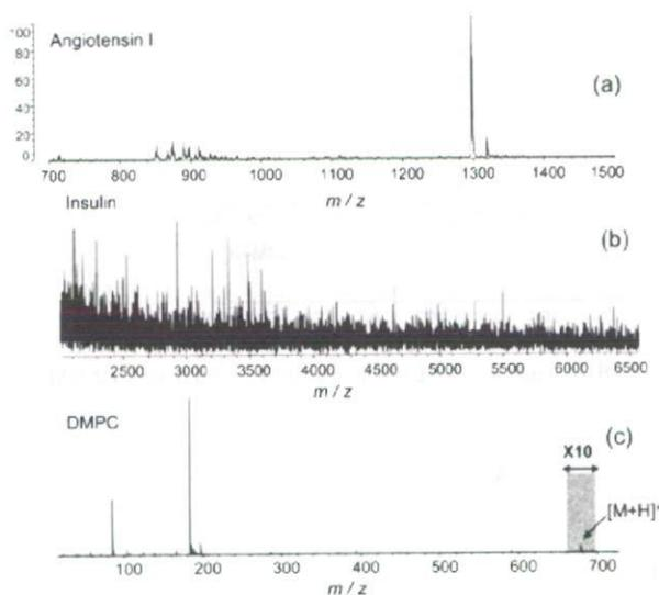
**Figure 7.** The mass spectra of (a) angiotensin I (5 pmol), (b) human insulin (5 pmol), and (c) DMPC (0.2 mg/mL, 0.5 mL) obtained from SALDI-MS with spherical Pt nanoparticles. The peak intensity,  $[M + H]^+$  is expanded by ten times.
