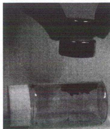
Fig. 4. Image of freeze-dried powder of iron oxide nanoparticles under a 1.1 T magnet ( $\text{FeCl}_3 \cdot 6\text{H}_2\text{O}$ : 175 mg).
