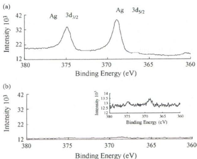
Fig. 4. X-ray photoelectron spectroscopic spectra of (a) Si-OH covered Si surface and (b) TTCl-SAM covered Si surface after their immersion into the dispersion of cationic Ag nanoparticles. Inset of (b), enlarged image.
