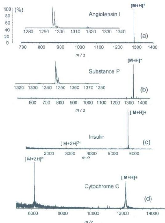
**Figure 2.** The mass spectra of (a) angiotensin I (500 fmol), (b) substance P (500 fmol), (c) human insulin (800 fmol), and (d) cytochrome C (5 pmol) obtained from Pt nanoflowers as the SALDI-MS.
