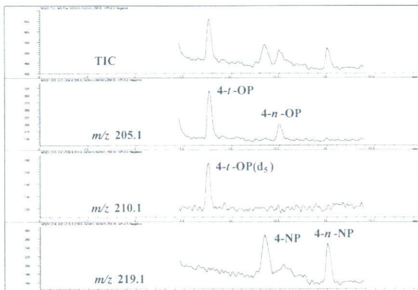
Fig. 1 Typical LC/ESI/MS-SIM chromatograms of standard mixture (1 ng/mL.)
