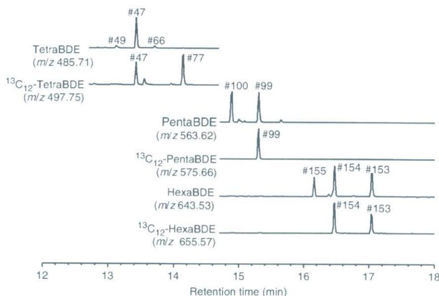
Figure 1. Chromatograms of PBDEs in deep-sea shark liver oil using GC/MS based on the isotope dilution method.
