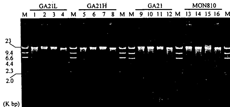
Fig. 1. Agarose gel electrophoresis of DNAs extracted from four powder samples including GA21H*, GA21L**, GA21 and MON810. Lane M, molecular marker \lambda Hind III; lanes 1, 5, 9 and 13, DNAs extracted using the maxi method; lanes 2, 6, 10 and 14, DNAs extracted using the mini method; lanes 3, 7, 11 and 15, DNAs extracted using the CTAB method; lanes 4, 8, 12 and 16, DNAs extracted using the WIZARD method.
