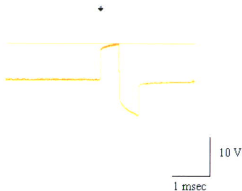
Figure 2. Photograph of oscilloscope monitor showing voltage between the active and the reference electrode. With biphasic rectangular pulse currents, the voltage increases slowly because of the effect of capacitance.
