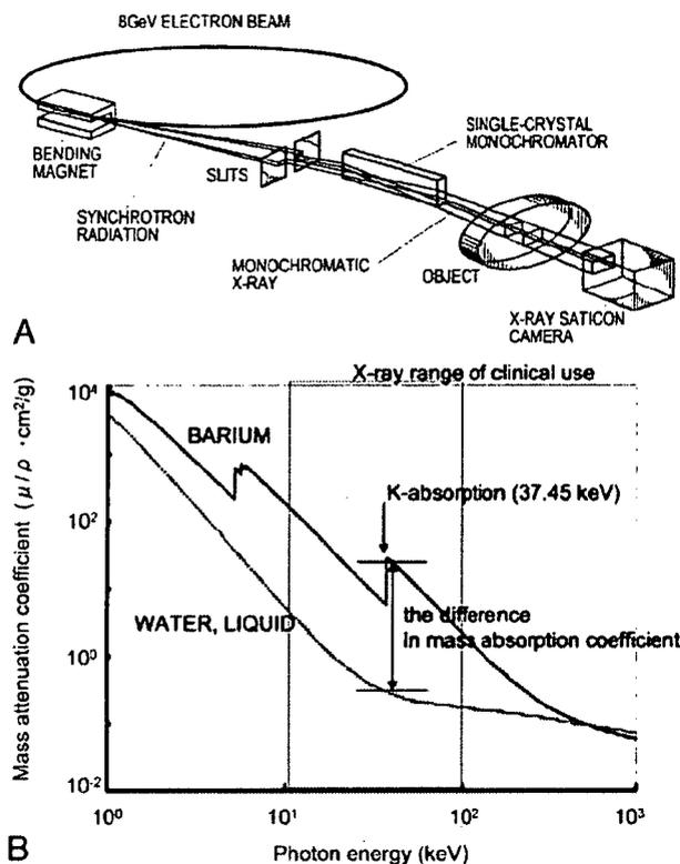
**Fig 1.** Schematic depiction of the monochromatic SR system. *A*, Illustration of the experimental arrangement for SR microangiography at BL28B2. *B*, Photon mass attenuation coefficient of barium (blue line) and liquid water (red line). Monochromatic x-ray energy is adjusted to 37.5 keV, just above the barium K-edge energy to produce the highest contrast image.
