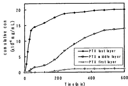
Fig. 7. Release profiles of PTX at different location from polymeric hydrogel multilayer of PMBV60(5.0 wt%) and PVA(1.5 wt%) in PBS+0.1 % Tween 20. Number of multilayer is the same as 6.
