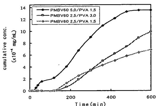
Fig. 6. Release profiles of PTX at the same location (middle in multilayer) from different polymer concentrations in PBS+0.1 % Tween 20
