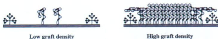
Fig. 11. Schematic representation of possible orientation of PMPC brushes grown from nanopores having different graft density.
