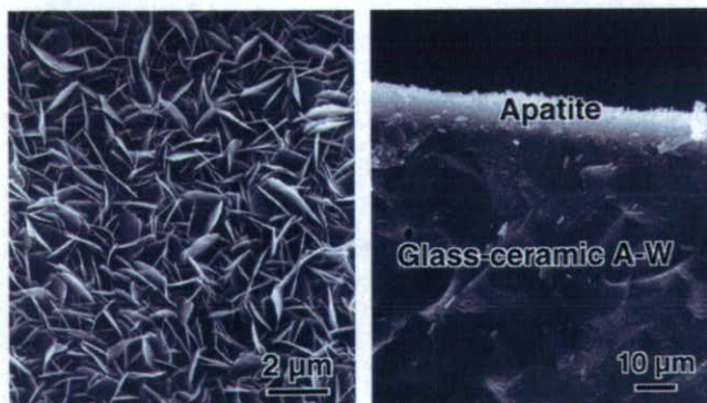
Fig. 1. Scanning electron micrograph of surface (left) and cross section (right) of apatite layer formed on glass-ceramic A-W in SBF [11].
