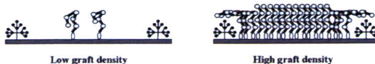
Fig. 11. Schematic representation of possible orientation of PMPC brushes grown from nanopores having different graft density.
