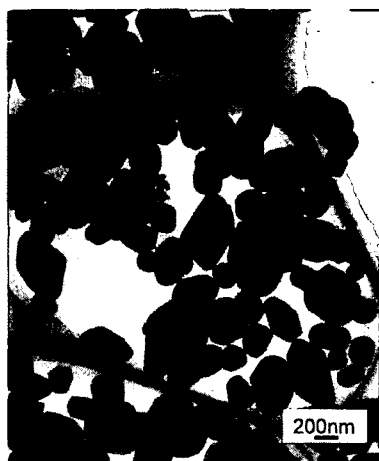
Fig. 1 Transmission electron micrograph of the as-received \text{TiO}_2 particles
