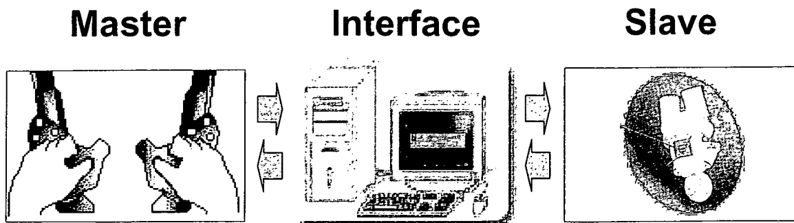
Fig. 1. Overview of the robotic surgery system. This system consists of a master controller, interface, and a slave manipulator. Input from the master controller is fed to the slave manipulator through the interface
