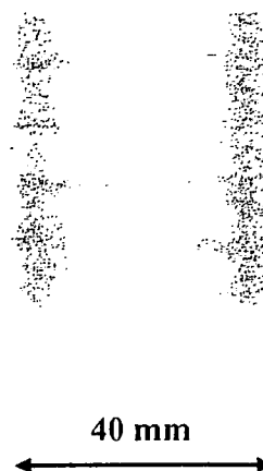
Fig. 5. Radiogram of a 200- \mu\text{m} -diameter tungsten wire coiled around a pipe made of polymethyl methacrylate.
