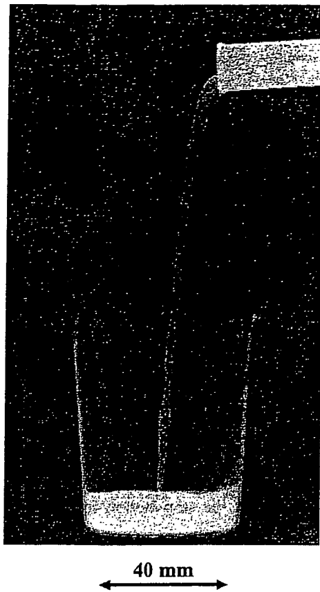
Fig. 10 Radiogram of water falling into polypropylene beaker from glass test tube.
