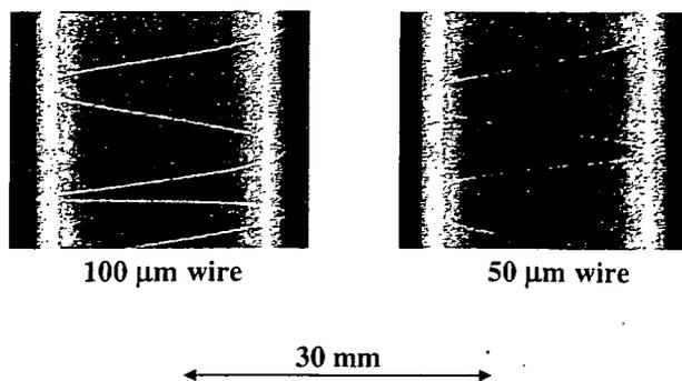
Fig. 8. Radiograms of tungsten wires of 50 and 100  $\mu$ m diameter coiled around a pipe made of polymethyl methacrylate with tube voltage of 25 kV and exposure time of 20 s.
