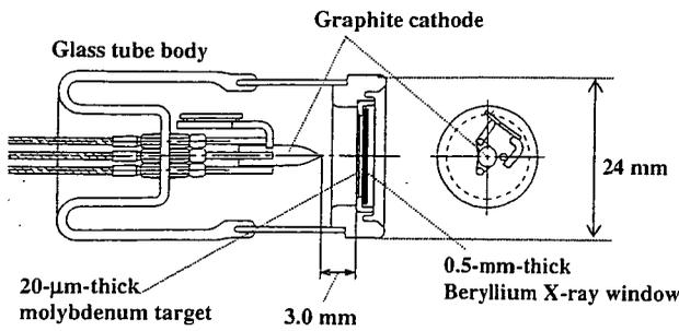
Fig. 2. Structure of X-ray tube.
