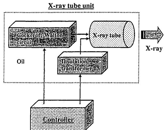
Fig. 1. Block diagram of compact X-ray generator with cerium-target radiation tube, which is used particularly for K-edge angiography using iodine-based contrast media.
