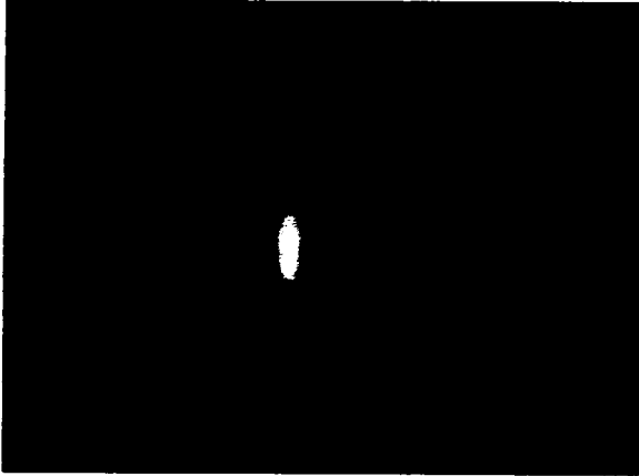
Figure 6: Beam profile at just after accelerating structure observed by luminescence screen. The energy of the electron beam is measured by bending magnet and is about 22 MeV,
