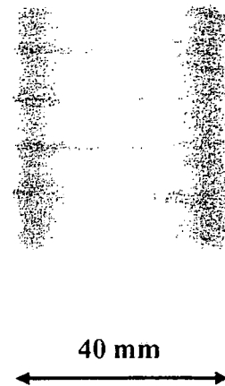
Fig. 5. Radiogram of a 200- \mu\text{m} -diameter tungsten wire coiled around a pipe made of polymethyl methacrylate.
