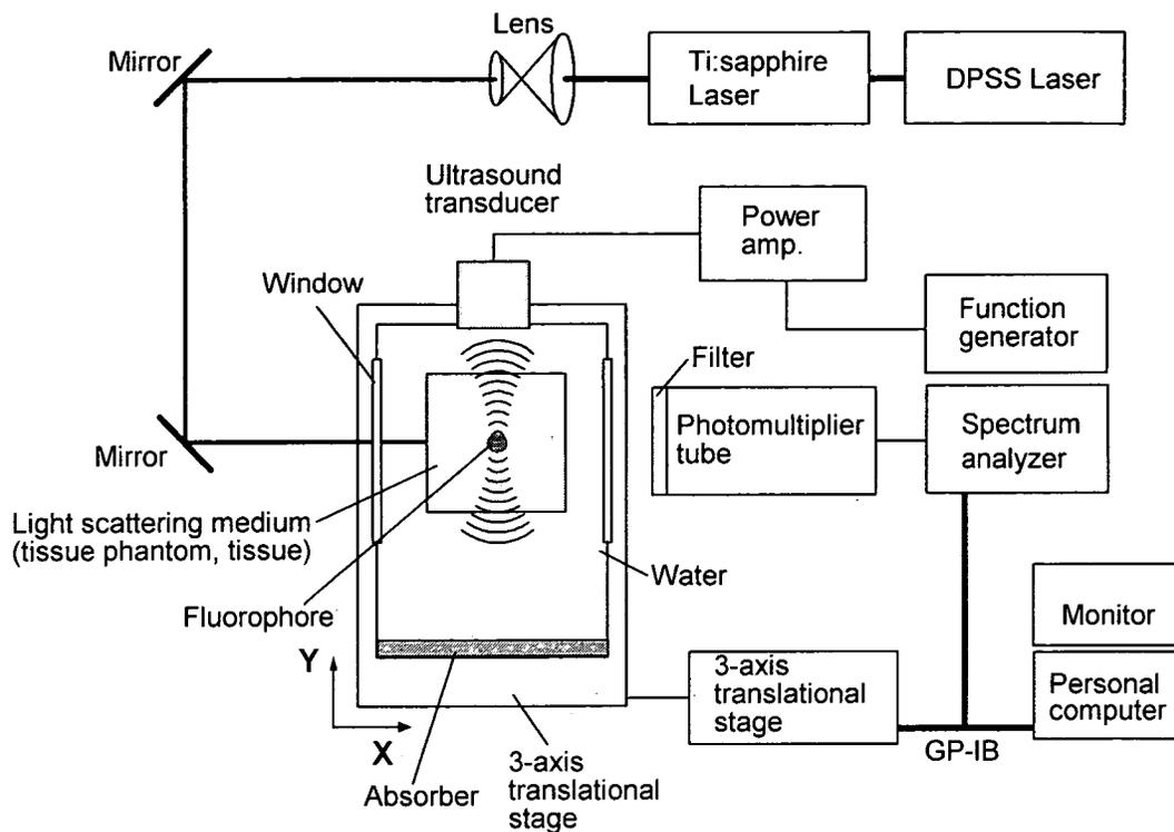
Fig. 1. Schematic of the experimental setup. A water tank equipped with an ultrasound transducer is set on the X-Y-Z auto-stage; a tissue phantom is fixed in place without touching the water tank.
