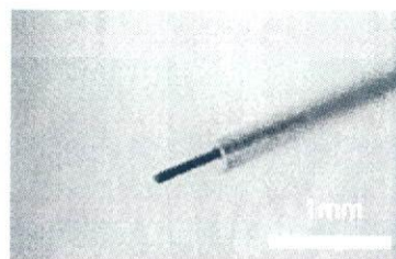
(a) Shape memory alloy fibre (D=100µm) covered with the silicone tubing
