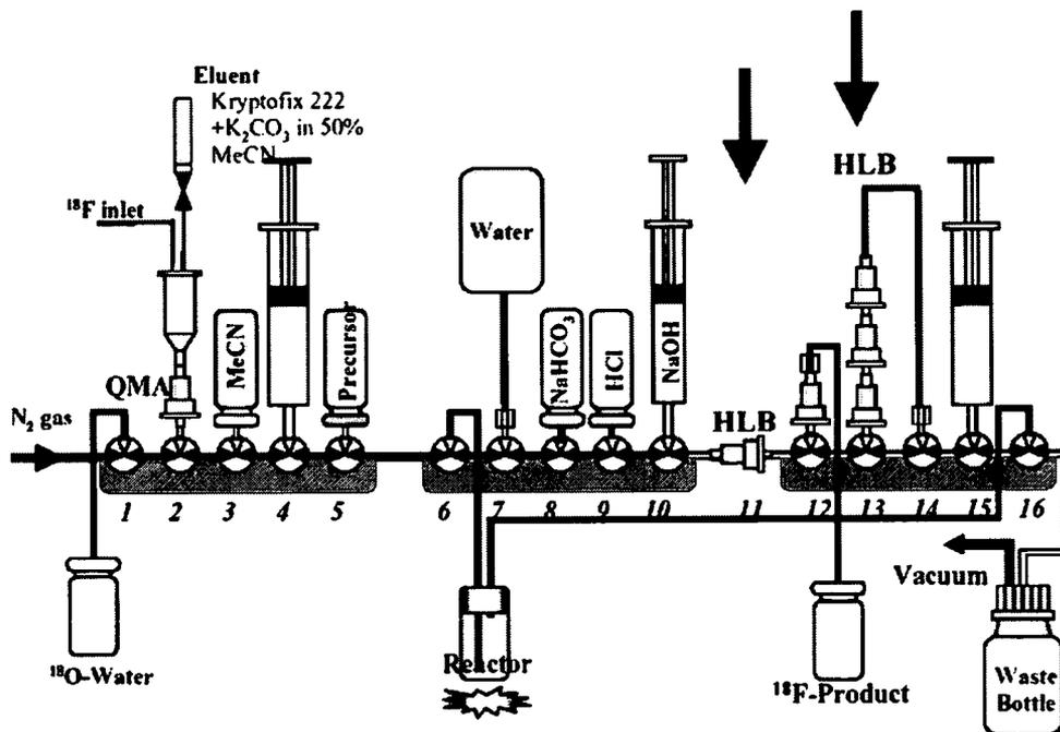
Fig. 2. Schematic diagram of TRACERlab MX<sub>FDG</sub> for the preparation of sodium [ $^{18}\text{F}$ ]fluoroacetate. Instead of Sep-Pak C-18 cartridges, one Oasis HLB Plus cartridge was placed at position 11 and three at position 13.
