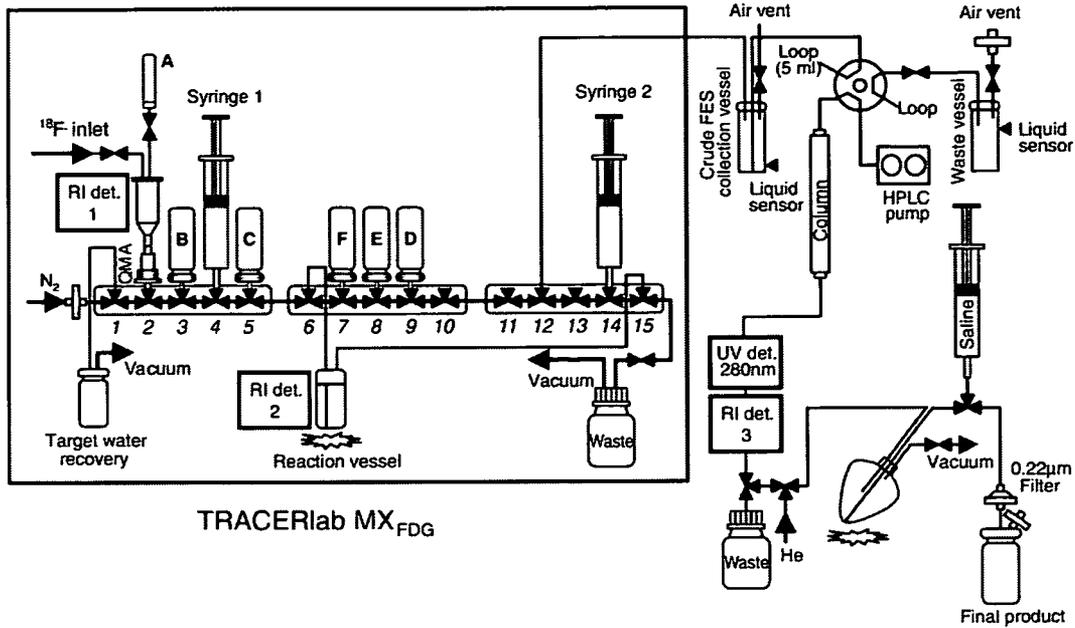
Fig. 2. Schematic diagram of the [ $^{18}\text{F}$ ]FES preparation system for clinical use.
