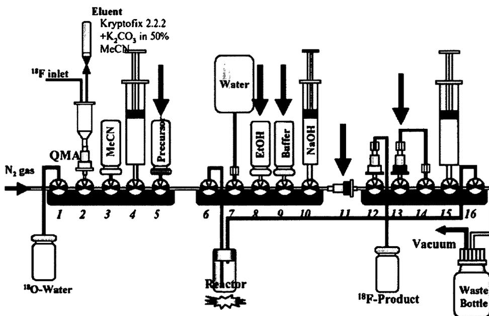
Fig. 1. Schematic diagram of TRACERlab MX<sub>FDG</sub> for the preparation of [<sup>18</sup>F]FDG. One Sep-Pak C-18 cartridge was placed at position 11 and another at position 13. The arrows indicate the parts to be replaced for the preparation of sodium [<sup>18</sup>F]fluoroacetate.
