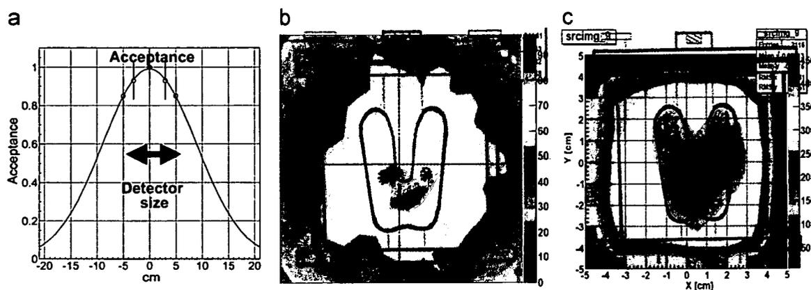
Fig. 5. (a) Acceptance of the detector, in which horizontal axis is an arbitrary unit. (b, c) are the images of the phantom of the human thyroid gland filled with  $^{131}\text{I}$  (364 keV) before and after applying the acceptance correction, respectively. The phantom was set on the 20 cm front from the center of the ETCC.
