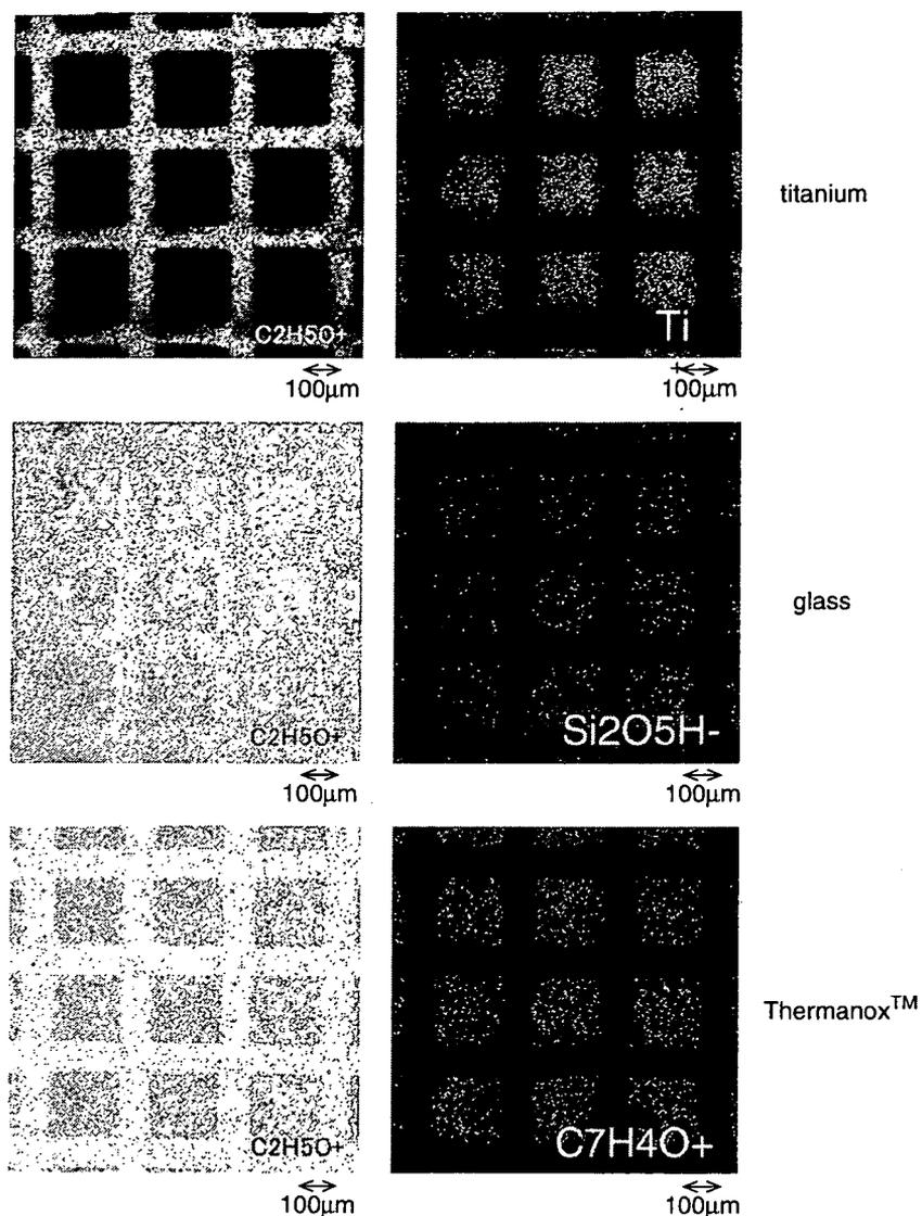
Fig. 5. TOF-SIMS image of PEG-micropatterned titanium, glass and Thermanox™.
