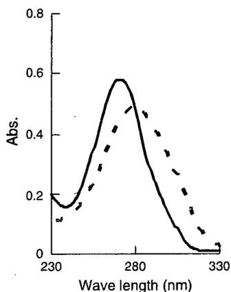
Fig. 3. UV spectrum of 4-azidoaniline hydrochloride ( $9.2 \mu\text{g ml}^{-1}$ , broken line) and photoreactive PEG (0.1 wt.% (the content of azidophenyl groups is  $10.5 \mu\text{g ml}^{-1}$ ), solid line).
