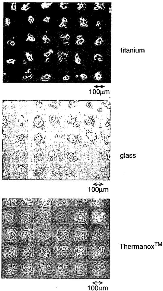
Fig. 9. Adhesion of COS-7 cells on micropattern photoimmobilized PEG on titanium, glass and Thermanox™.
