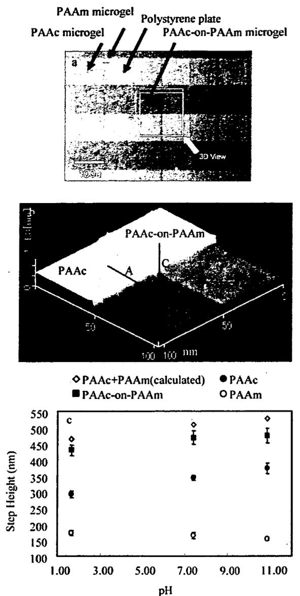
**Figure 2.** (a) Optical micrograph and (b) 3D topographic image of scanning probe microscopy (SPM) of a grid pattern of the PAAc-on-PAAM microgel network and (c) changes in the heights of the areas of PAAc, PAAc, and PAAc-PAAM microgels with changes in pH. The average value and the standard deviation for  $n = 5$ . The calculated height is the sum of the heights of PAAc and PAAm microgels.
