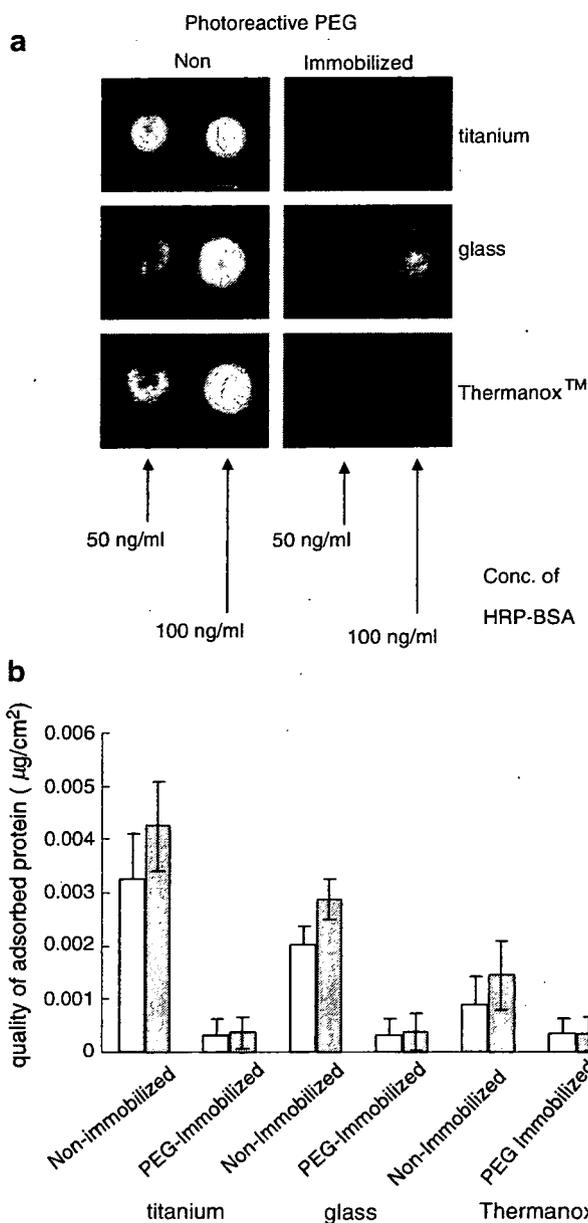
Fig. 8. (a) Chemiluminescence of HRP-BSA on non-immobilized and PEG-photoimmobilized titanium, glass, and Thermanox™. (b) The amount of HRP-BSA on non-immobilized and PEG-photoimmobilized titanium, glass, and Thermanox™. Open and closed columns indicate 50 and 100 ng ml<sup>-1</sup> of protein concentrations, respectively.
