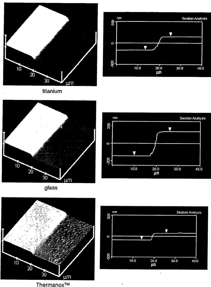
Fig. 6. AFM images of PEG micropatterned on titanium, glass and Thermanox™.
