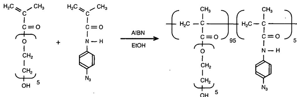
Fig. 1. Synthetic scheme for producing photoreactive PEG.
