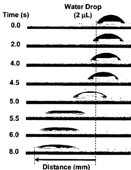
**Figure 5.** The movement of a water drop and its related equation. Water drop size = 2 μL.
