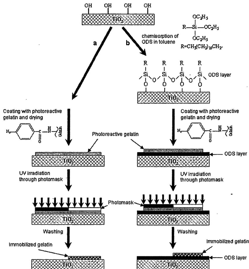
**Figure 1.** Schematic illustration of the pattern-immobilization of photoreactive gelatin on (a) titan and (b) titan modified with ODS.
