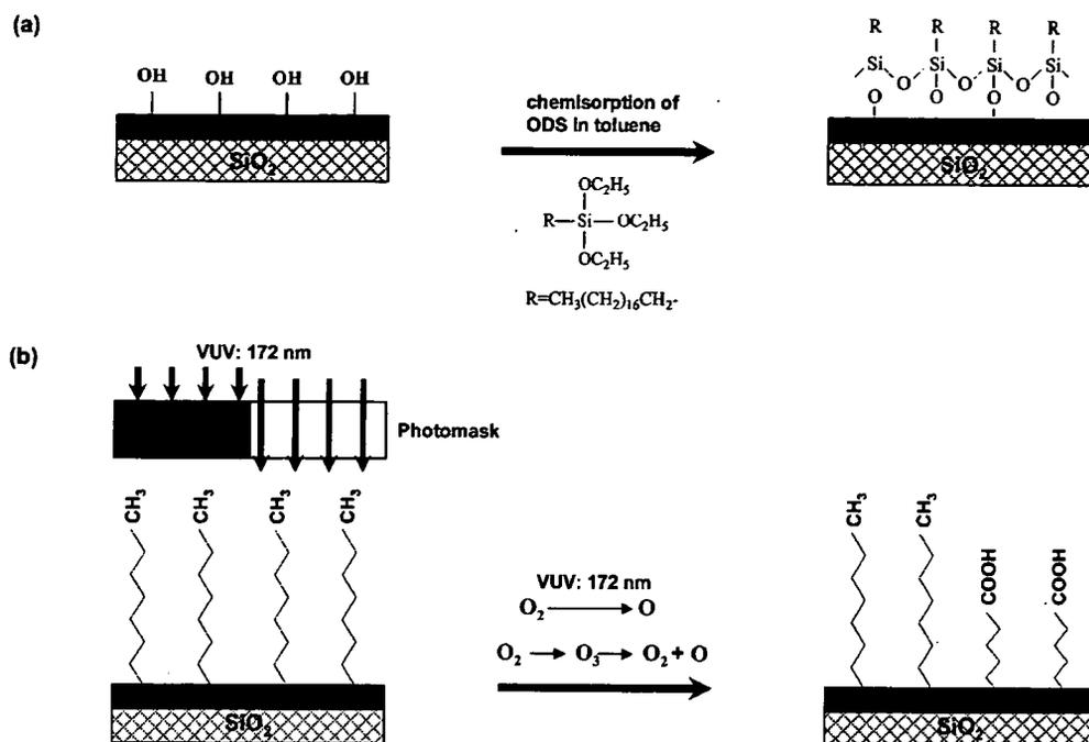
**Figure 1.** Preparation of surface gradient by photodegradation. (a) Surface treatment of glass plates by a silane coupling reaction. (b) Excitation of the surface molecules by VUV irradiation and oxygen molecules cleaved by the VUV.
