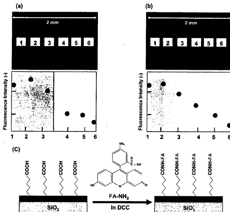
**Figure 4.** (a) Fluorescence microscopy of a pattern surface and (b) a gradient surface. The surface was labeled with 5-aminofluorescein (FA-NH<sub>2</sub>), which targeted the VUV irradiated regions on the surface. Luminance = 1 mW/cm<sup>2</sup> and exposure time = 20 s.
