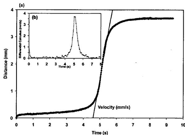
**Figure 6.** (a) Position of a droplet with nominal volume = 2 μL plotted against the transverse time, on a surface prepared such that irradiation energy and slide movement rate were 1.2 mW/cm<sup>2</sup> and 0.05 mm/s, respectively. The velocity of the water droplet was determined by the sharpest slope. (b) Time dependence of the differential of a.
