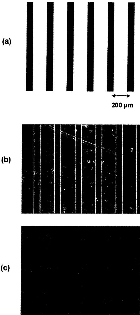
Figure 4. Optical microscopic micrographs of (a) photomask and immobilized pattern of photoreactive gelatin in a striped pattern on (b)  $\text{TiO}_2$  and (c)  $\text{TiO}_2\text{-ODS}$ . [Color figure can be viewed in the online issue, which is available at [www.interscience.wiley.com](http://www.interscience.wiley.com).]
