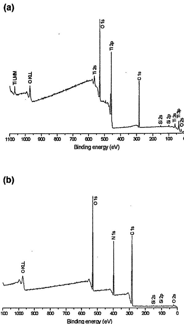
Figure 3. XPS wide scan spectrum of titanium treated (a) with ODS and (b) with photoreactive gelatin.
