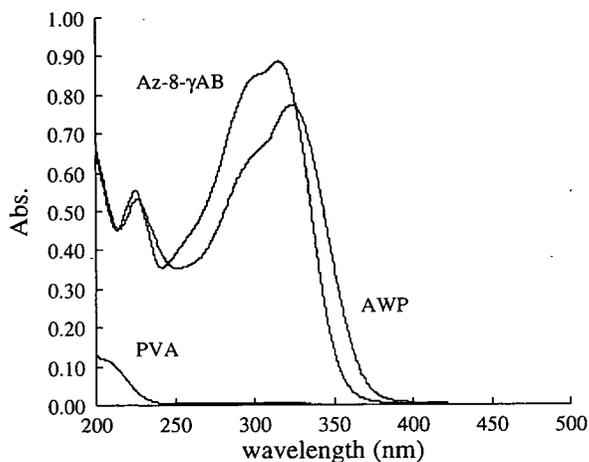
Fig. 4. UV spectra of Az-8- $\gamma$ AB, polyvinylalcohol, and AWP.
