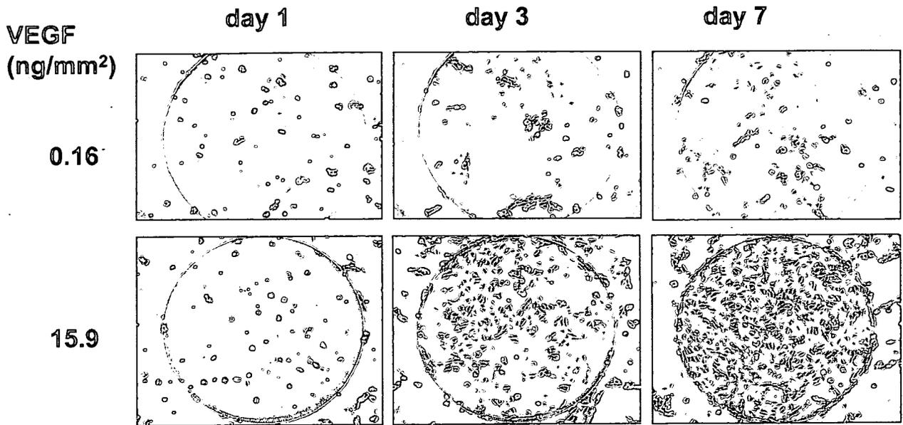
**Figure 3.** Phase-contrast micrographs of HUVECs cultured on tissue culture polystyrene dishes with different concentrations of immobilized VEGF. The immobilized region is in the center of each photo. The surface concentration of gelatin was  $15.9 \text{ ng/mm}^2$ .
