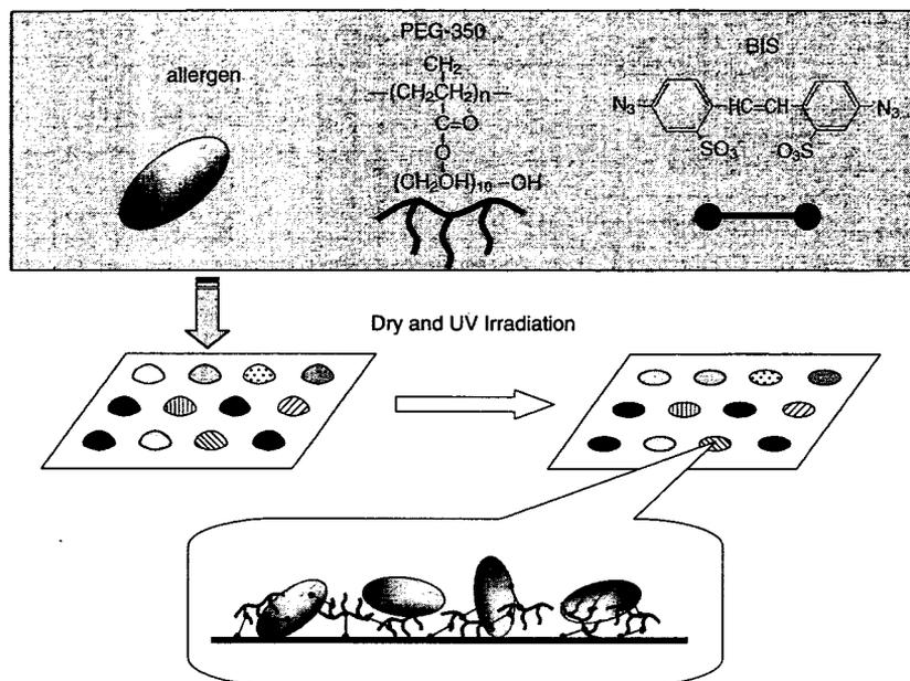
**Fig. 1** Illustration of the photo-immobilization method. Abbreviations: PEG-350, polymer carrying polyethylene glycol in the side chains; BIS, 4,4'-diazido-stilbene-2,2'-disulfonic acid disodium salt.
