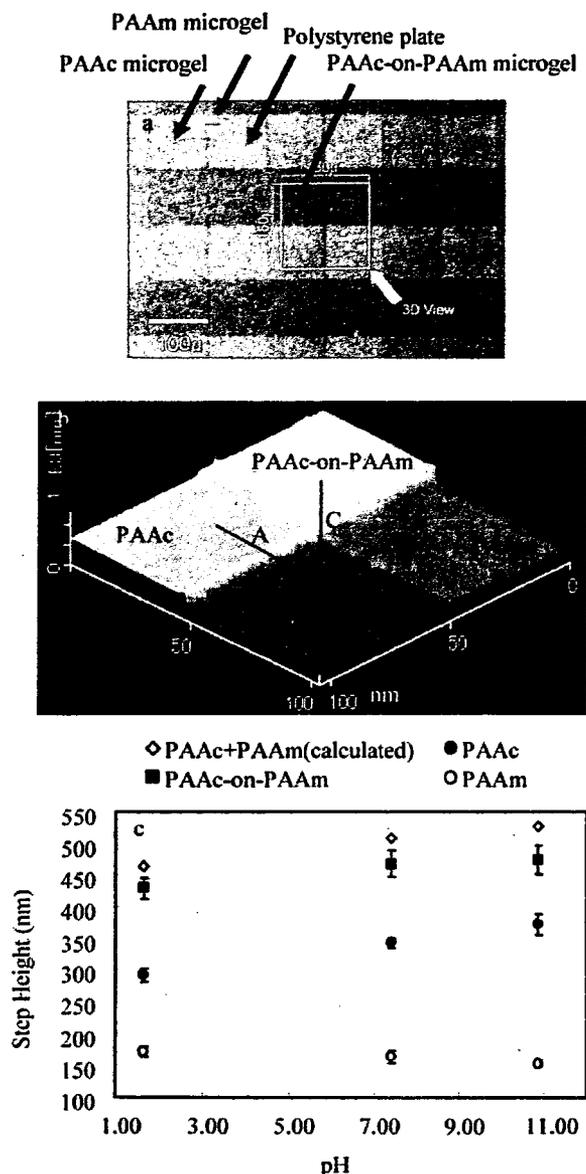
**Figure 2.** (a) Optical micrograph and (b) 3D topographic image of scanning probe microscopy (SPM) of a grid pattern of the PAAc-on-PAAm microgel network and (c) changes in the heights of the areas of PAAm, PAAc, and PAAc-PAAm microgels with changes in pH. The average value and the standard deviation for  $n = 5$ . The calculated height is the sum of the heights of PAAm and PAAc microgels.
