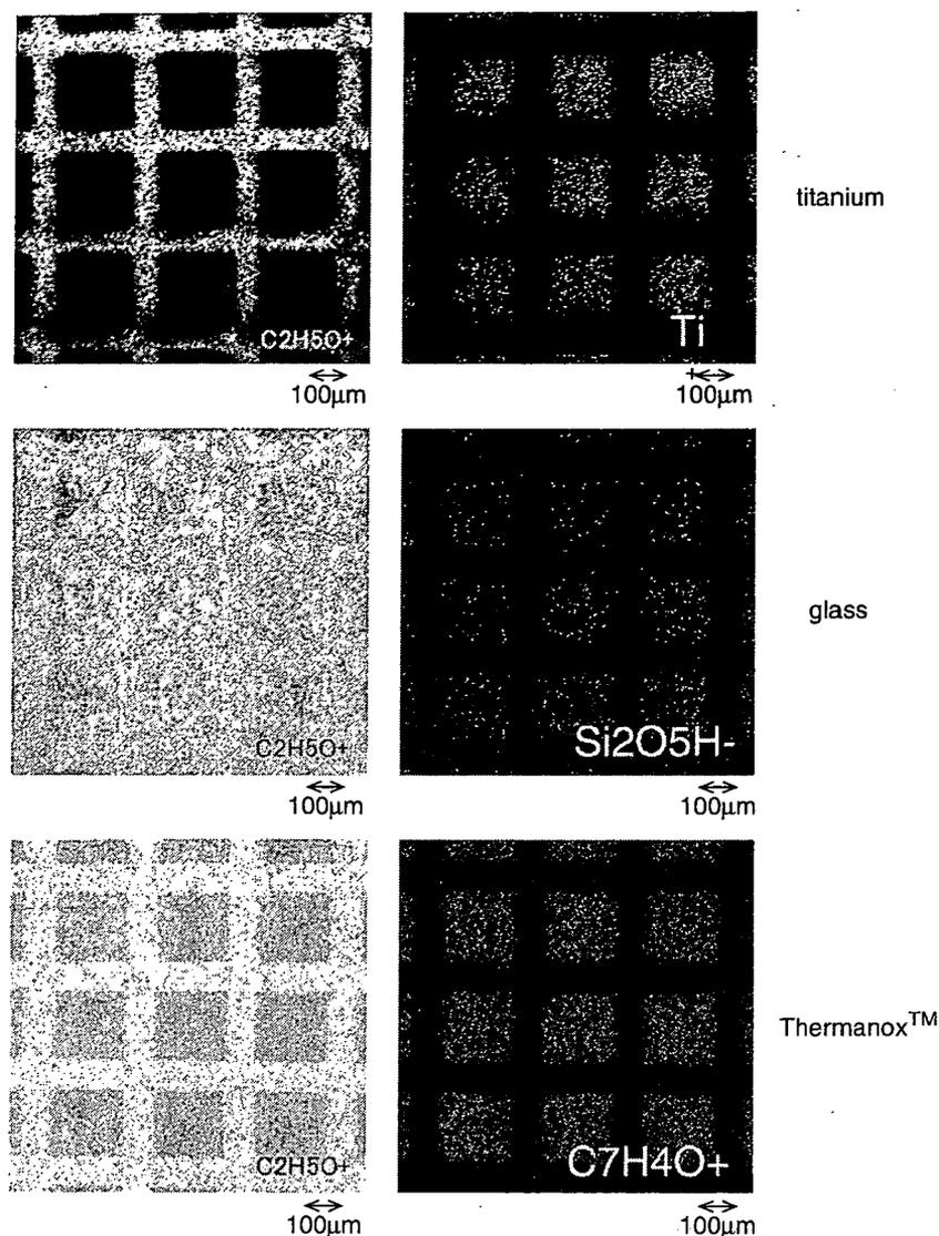
Fig. 5. TOF-SIMS image of PEG-micropatterned titanium, glass and Thermanox™.
