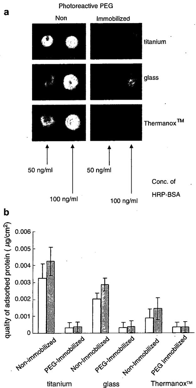
Fig. 8. (a) Chemiluminescence of HRP-BSA on non-immobilized and PEG-photoimmobilized titanium, glass, and Thermanox™. (b) The amount of HRP-BSA on non-immobilized and PEG-photoimmobilized titanium, glass, and Thermanox™. Open and closed columns indicate 50 and 100 ng ml<sup>-1</sup> of protein concentrations, respectively.
