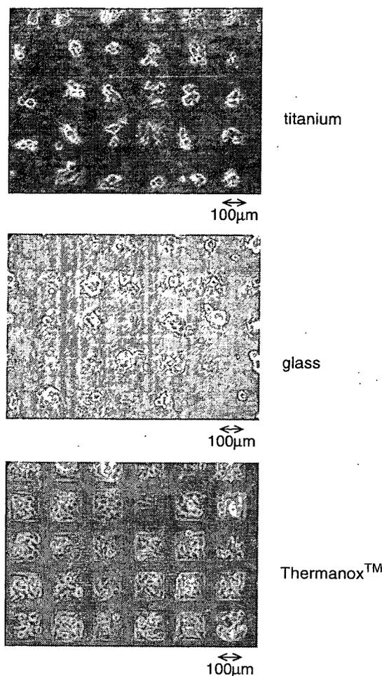
Fig. 9. Adhesion of COS-7 cells on micropattern photoimmobilized PEG on titanium, glass and Thermanox™.
