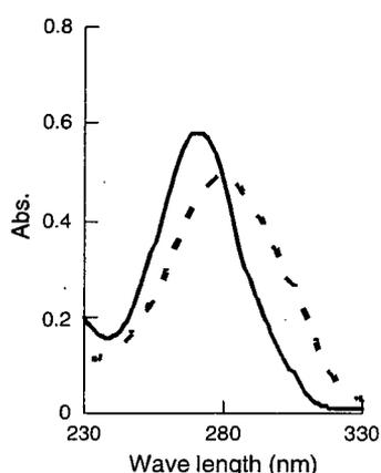
Fig. 3. UV spectrum of 4-azidoaniline hydrochloride ( $9.2 \mu\text{g ml}^{-1}$ , broken line) and photoreactive PEG ( $0.1 \text{ wt.}\%$  (the content of azidophenyl groups is  $10.5 \mu\text{g ml}^{-1}$ ), solid line).
