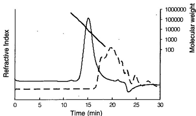
Fig. 2. Gel permeation chromatography of polymethacryl-PEG (broken line) and photoreactive PEG (solid line).
