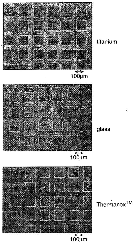
Fig. 4. Phase-contrast micrographs of micropatterned titanium, glass and Thermanox™ surfaces.
