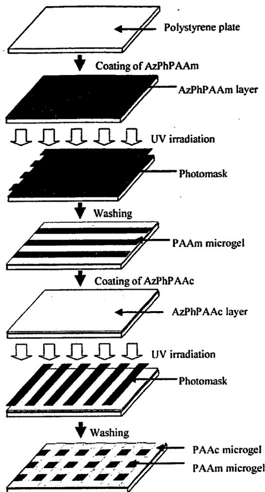
**Figure 1.** Photolithographic fabrication scheme of the grid pattern of microgel networks.
