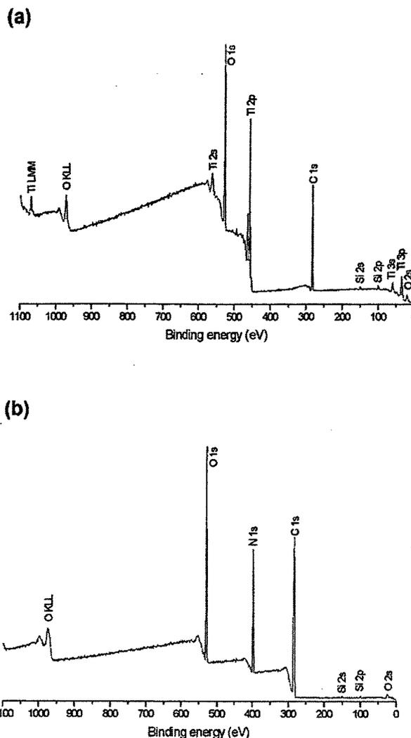
**Figure 3.** XPS wide scan spectrum of titanium treated (a) with ODS and (b) with photoreactive gelatin.
