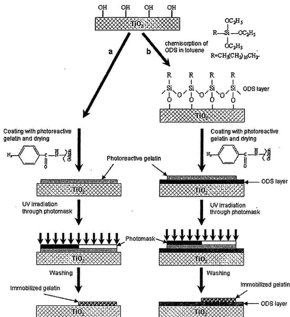
**Figure 1.** Schematic illustration of the pattern-immobilization of photoreactive gelatin on (a) titan and (b) titan modified with ODS.
