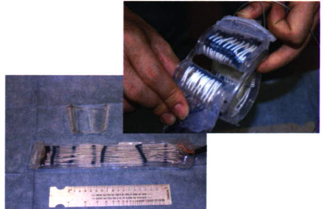
(b) Whole view of the myocardial assist device developed
