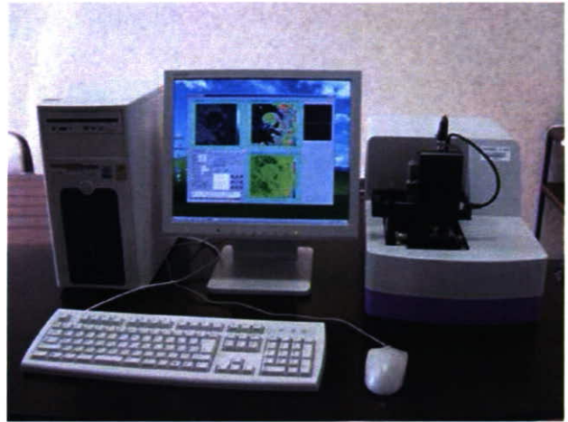
Figure 2. Appearance of the speed of sound microscopy.
