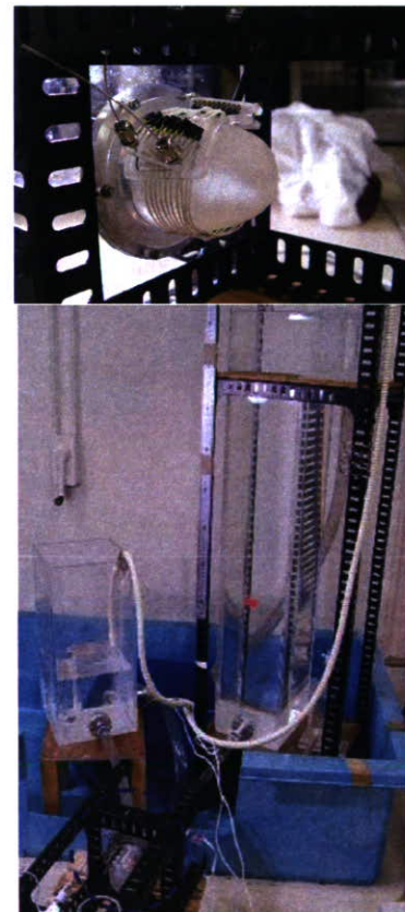
Fig. 3: Hydrodynamic examination of the artificial myocardium (top); the device was attached onto the silicone mock left ventricular model (bottom).
