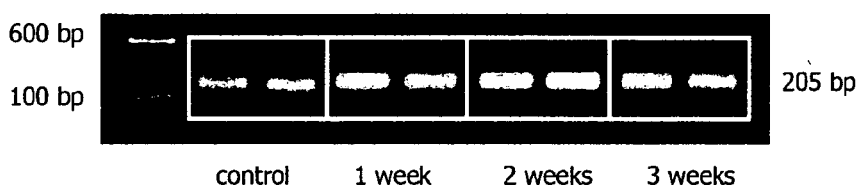
Fig. 5. Expression of the bFGF gene at 1, 2, and 3 weeks after gene transfer. Gel electrophoresis shows the location and density of the bands of the bFGF gene of tenocytes receiving exogenous bFGF and those in the control.
