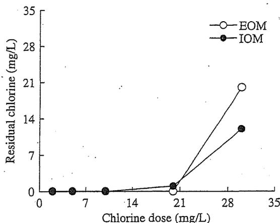
**Figure 3** The relationship between chlorine dose and residual chlorine after chlorination of EOM and IOM
