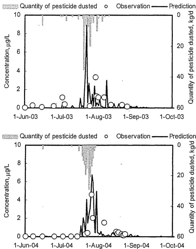
Figure 4 Comparison of observed time-series isoprothiolane concentrations with those predicted by the model.
