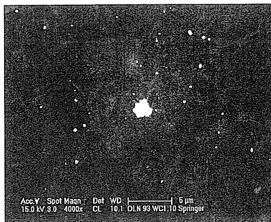
Fig. 4b: OLN 93 cells, incubated with 10 µg/ml WC NP for 1 h. BSE-detector image (4000×)
